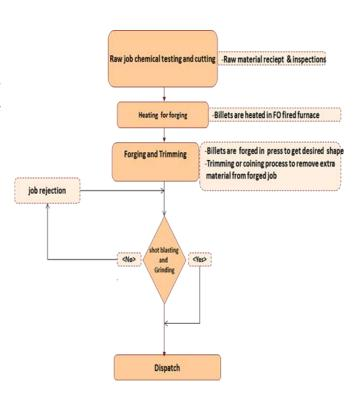
The major energy consuming equipments used were an FO-fired forging furnace and FO-fired heat treatment furnace, an electrical holding furnace, two electrical billet heating furnaces, and electrical motors associated with process equipment such as air compressor, pumps, etc.
