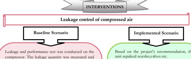
comes out to be 0.92 Nm3/min. The average operating power was 15 kW. As per the performance test of the compressor the free air discharge is 1.94 Nm<sup>3</sup>/min and the leakage quantity was 0.92 Nm3/min.
