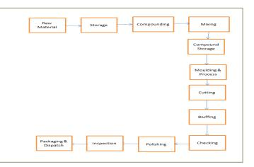
open mould cavity and then closing the mould. Thermo set materials are cured by an irreversible chemical reaction under heat and pressure. The result of this reaction is a highly cross-linked molecular structure. After curing the component is ready, it is inspected and finally dispatched
