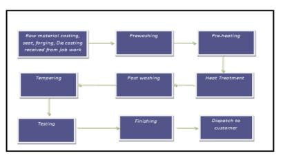
nitriding, hardening and quenching are done. The heat treated products are allowed to pass through water to remove excess oil sticking to the pieces. The pieces are sent to tempering furnace where there are further heat treated to get desired properties. The pieces are finally sent tested at different parameters and finished using bench grinder and shot blasting machine and finally dispatched.
