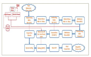
gun. These powder coated item goes for heat treatment in oven at 200°C.After heat treatment it is cleaned and inspected for quality. After quality testing finished product packed and stored for dispatch.
