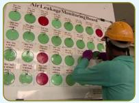
Leakage Monitoring. Personnel maintain an Air Leakage Monitoring Board that indicates the current status of compressed air leakages at the various pneumatic power presses and other machines.
