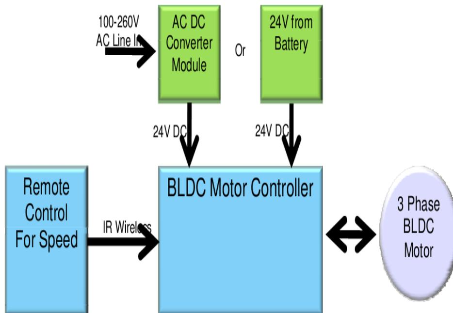
Figure 26: Schematic of BLDC fan
