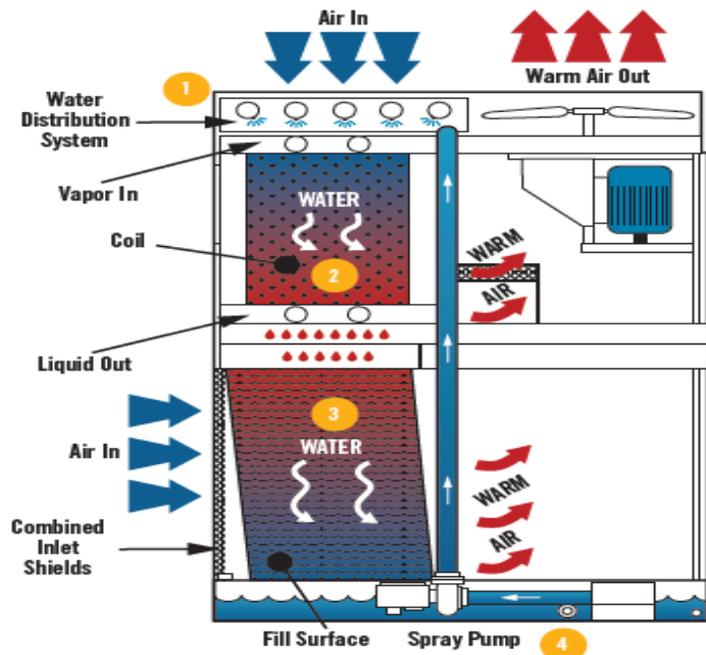
Figure 25: Evaporative condenser
