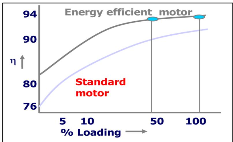
Figure 18: Loading Vs Efficiency curve
