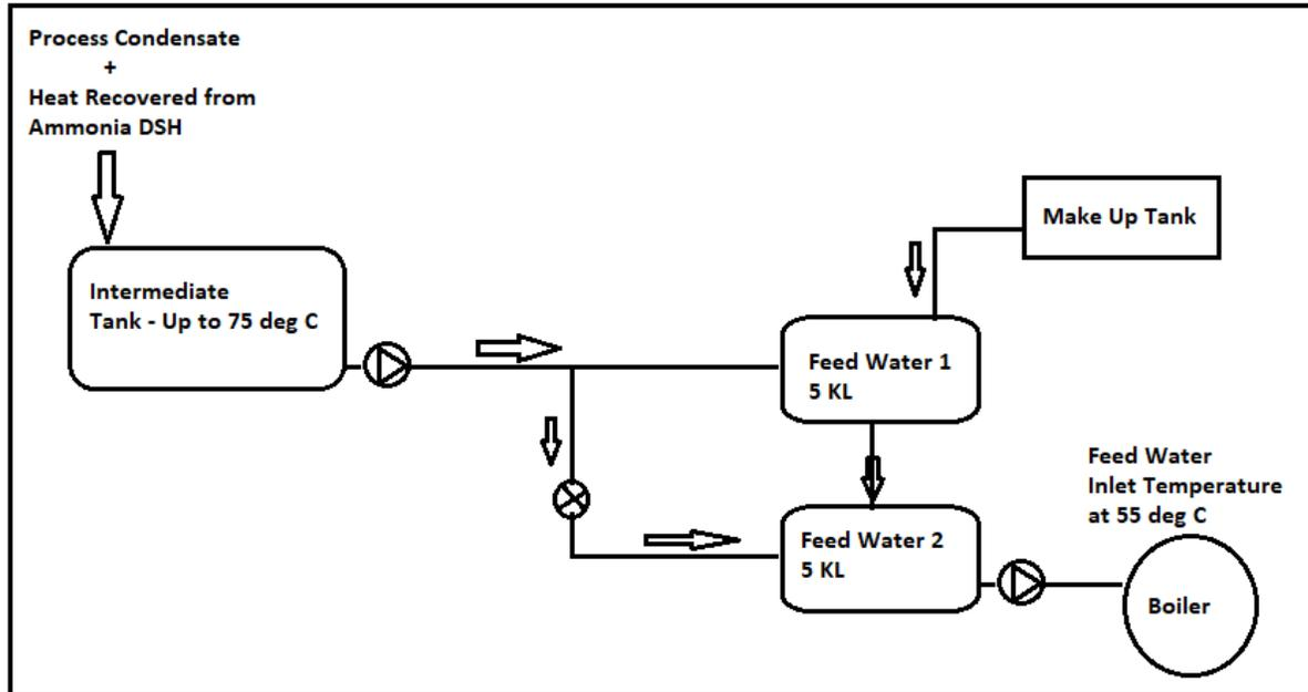
Figure 14: Schematic of hot water sources in the plant
