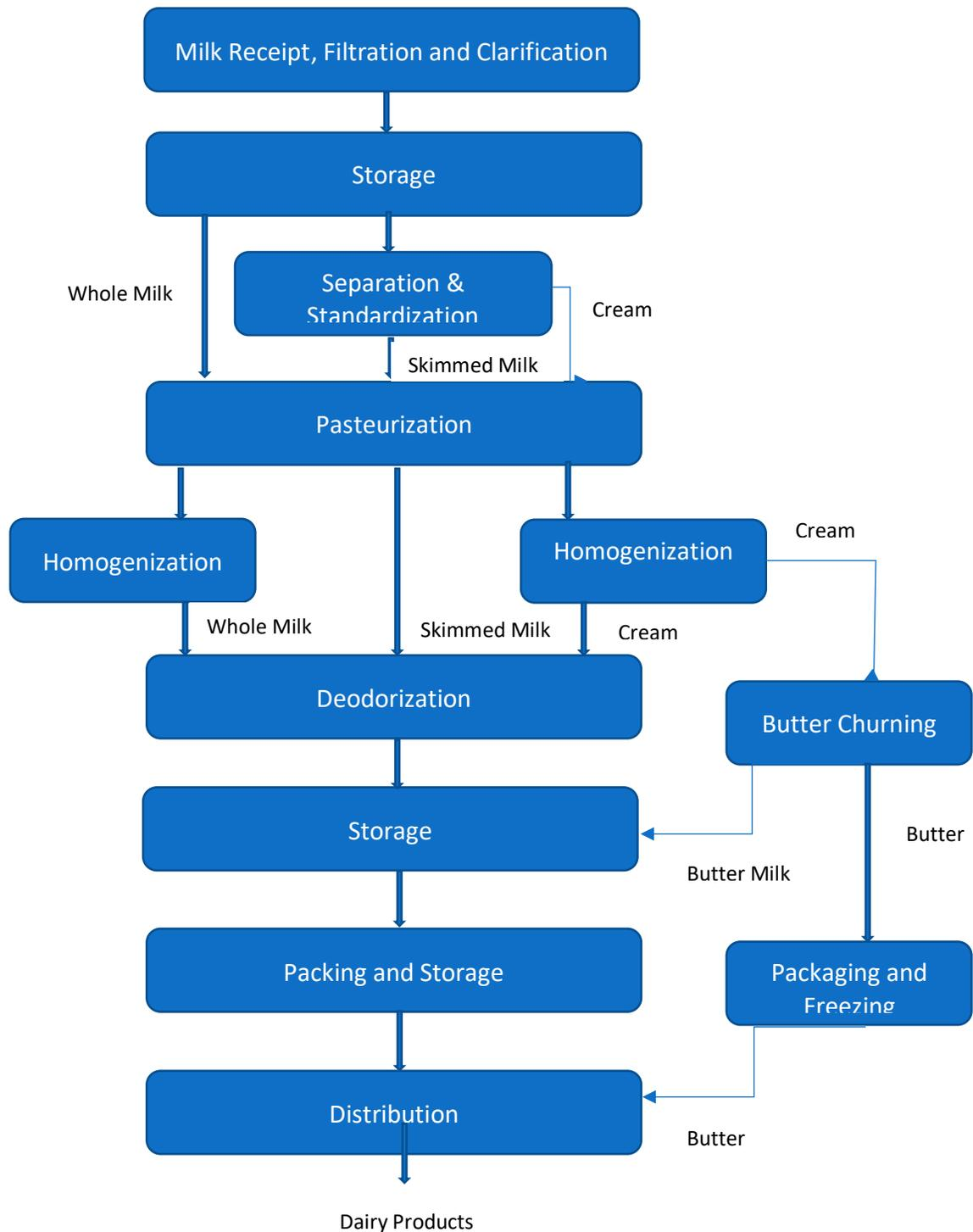
Figure 2: Typical process flow of Milk manufacturing
