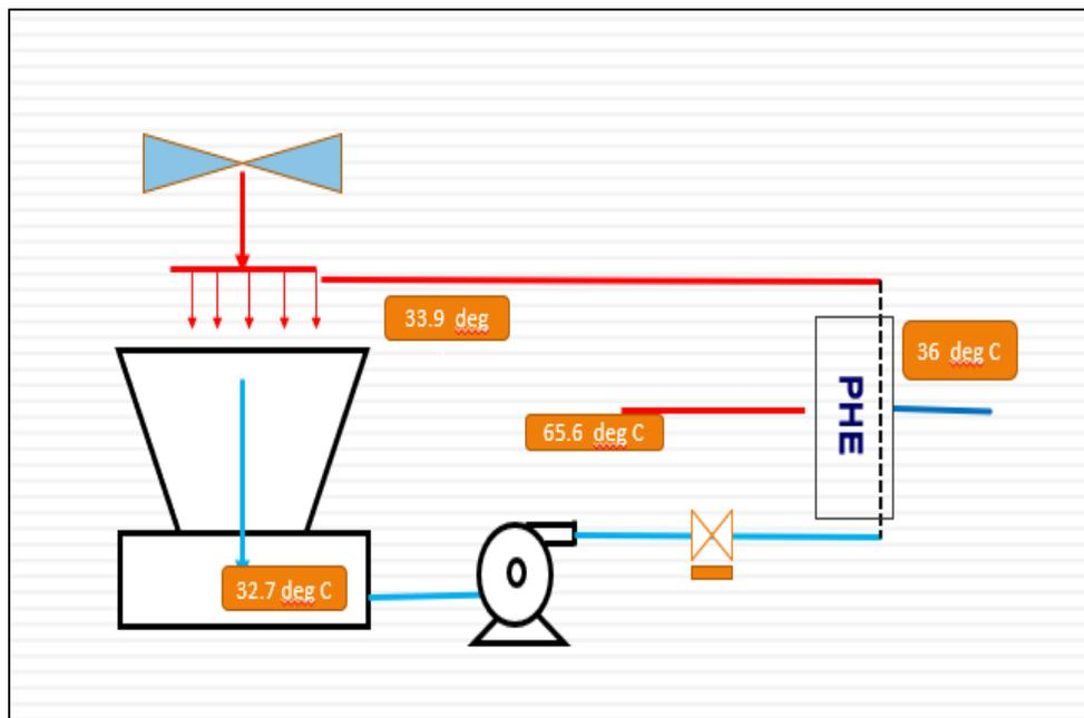
Figure 17: Schematic of PHE Condenser
