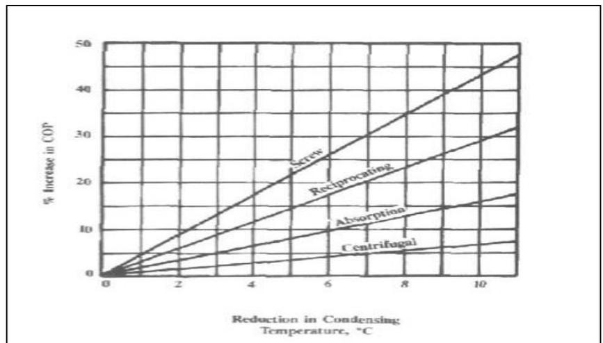
Figure 24: Effect of condensing temperature on COP
