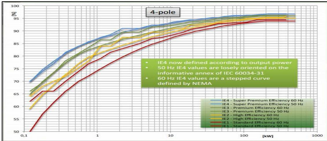
Figure 21: Losses in different classes of motors
