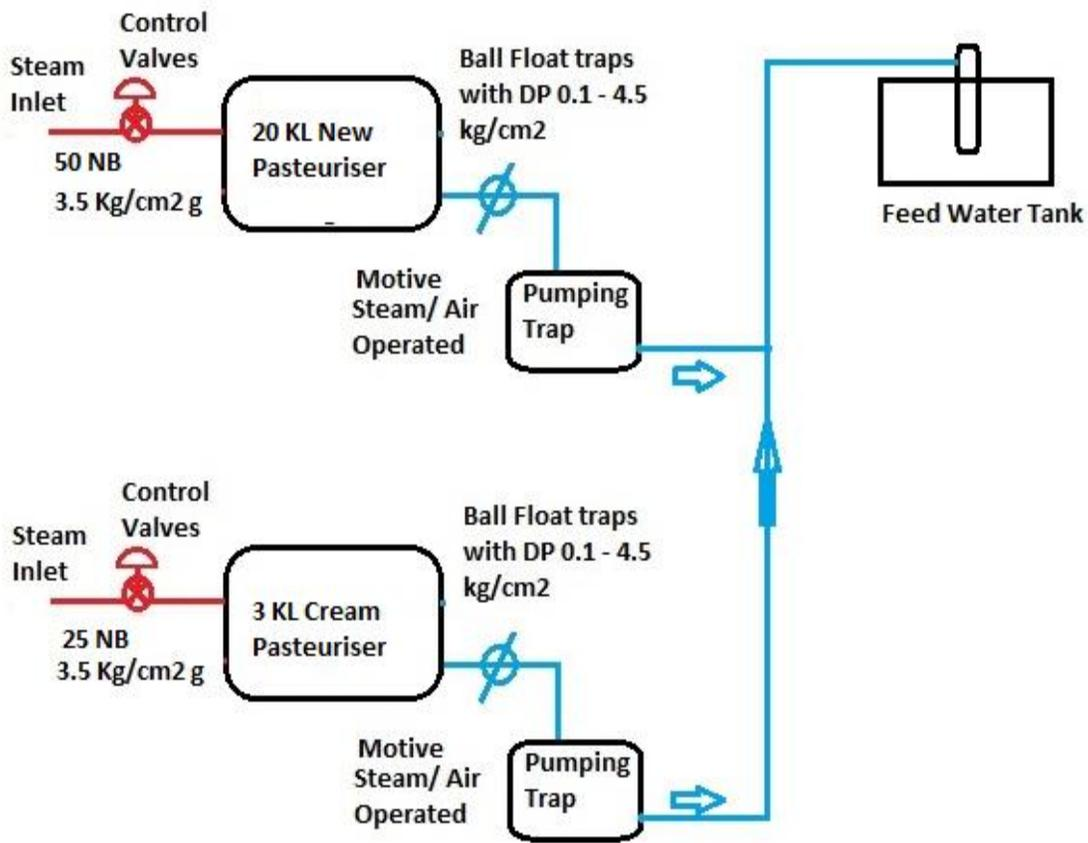
Figure 15: Schematic layout with trap installation
