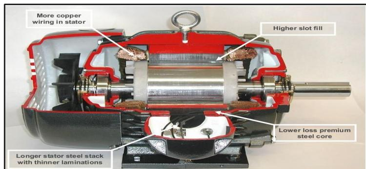
Figure 19: EE Motor features
