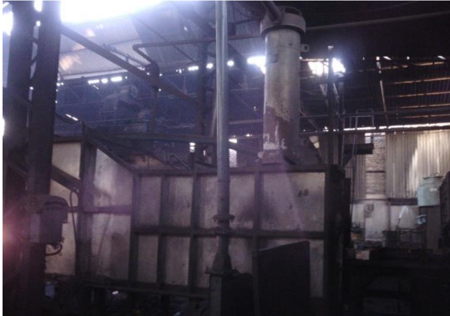
Figure 3: Forging furnace in a hand tool unit at Jalandhar
