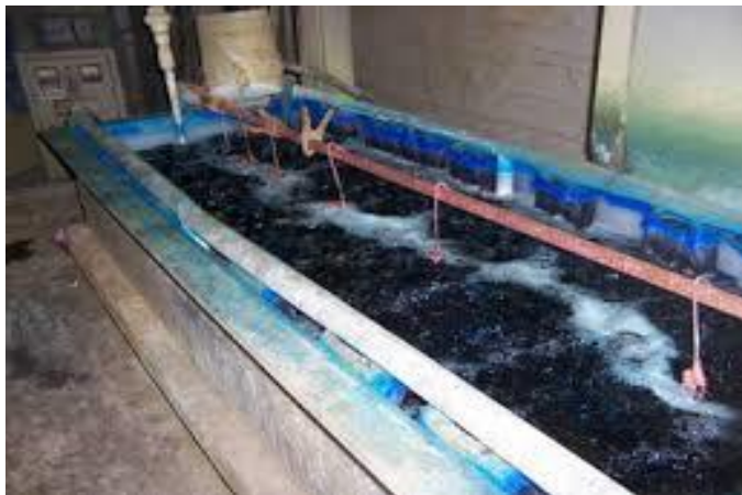
Figure 10: Electroplating bath in operation
