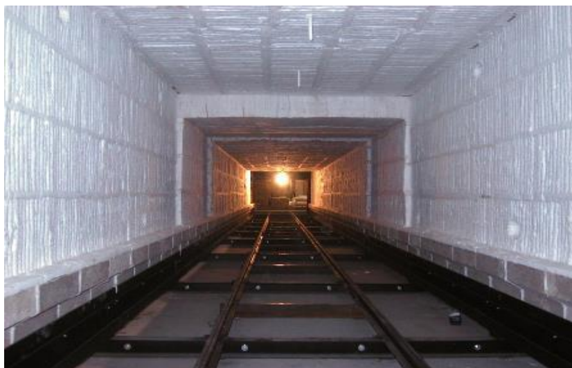
Figure 7: Good insulation in tunnel kiln
