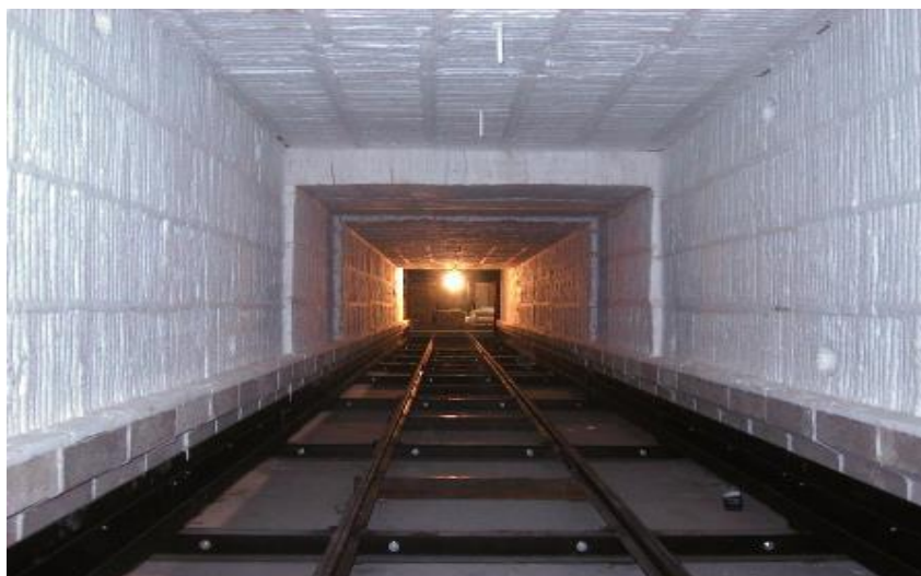
Figure 6: Good insulation in tunnel kiln
