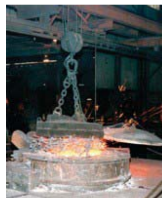
Figure 2.7: Overfilling of induction furnace crucible
