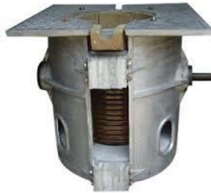
Figure 6.5: Induction furnace for brass melting
