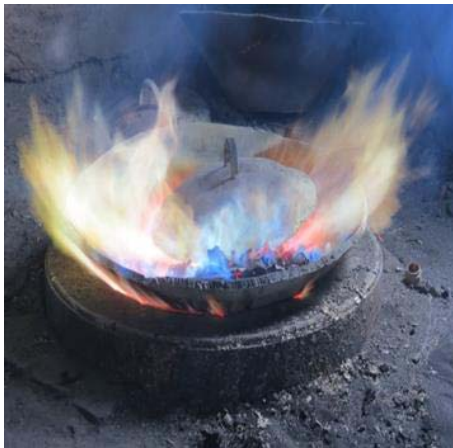
Figure 6.4: Conventional coal based pit furnace
