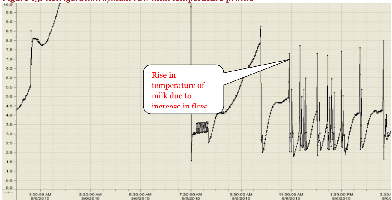
Figure 13: Refrigeration system raw milk temperature profile
