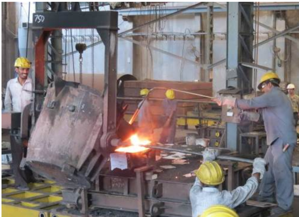
Figure 2.12: Pouring of molten metal to moulds
