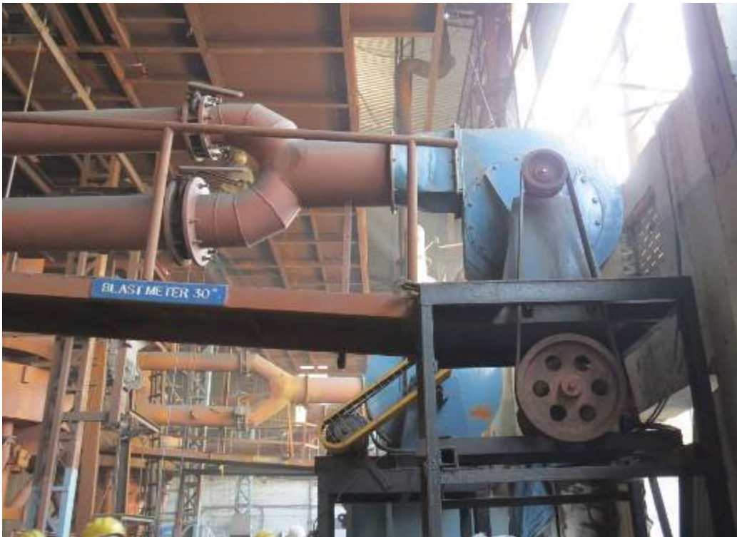
Figure 2.18: Blower to supply air for cupola operation
