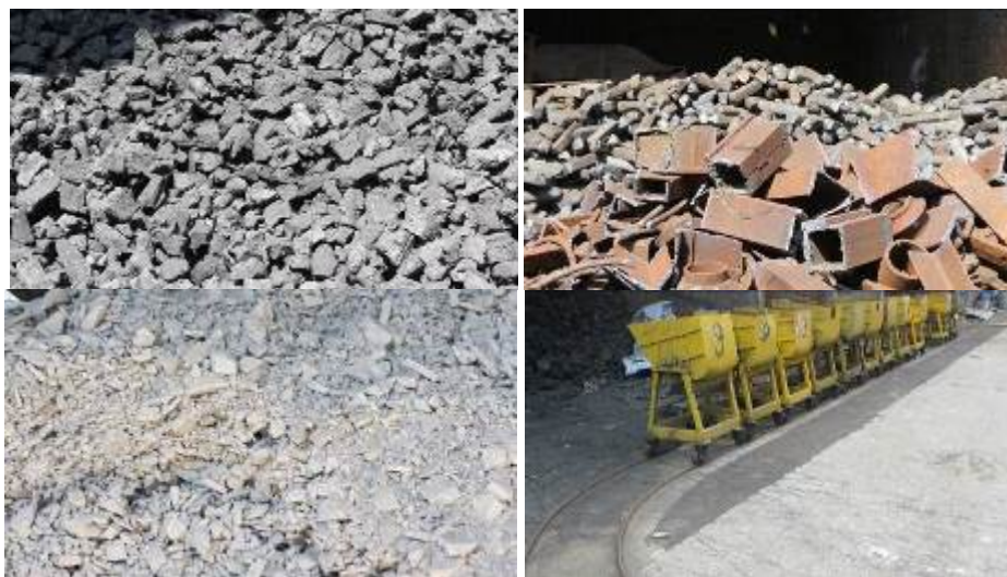
Figure 2.6: Coke, lime and raw material to be used in cupola
