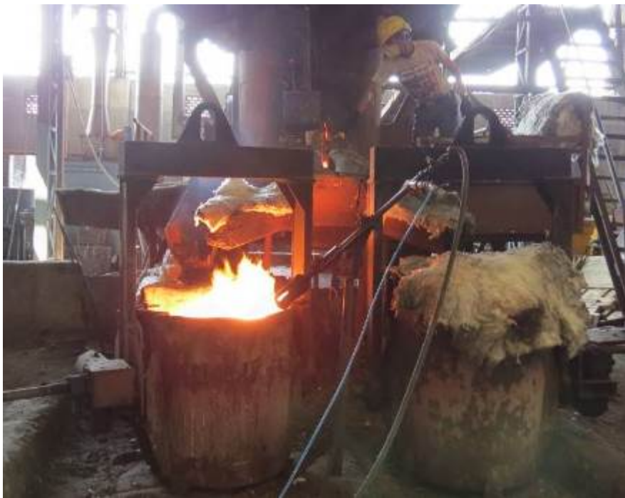
Figure 2.8: Preheating of ladle using diesel fired burner
