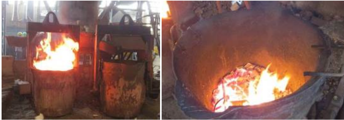
Figure 2.7: Preheating of ladle using firewood
