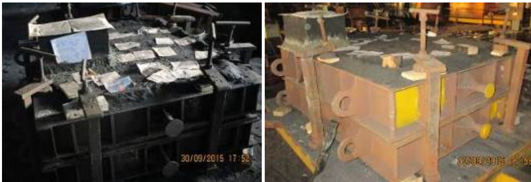
Figure 2.5: Moulds ready for pouring
