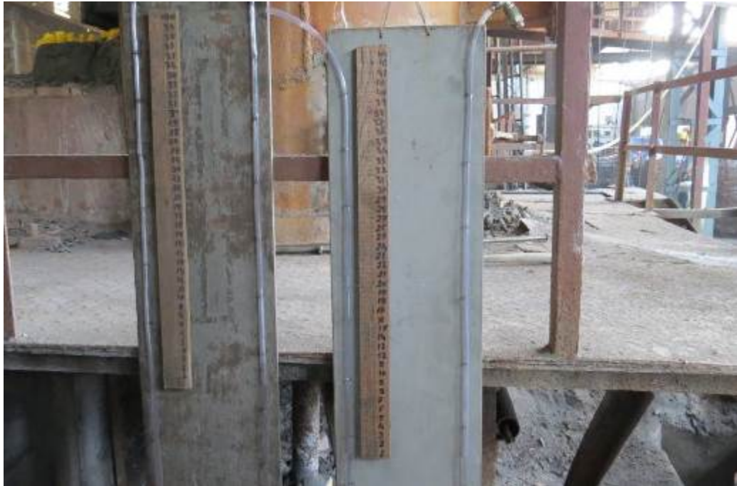
Figure 2.19: Manometer to measure air flow rate
