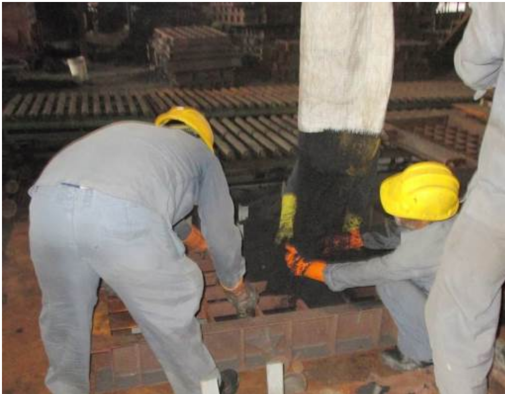
Figure 2.3: Moulding of sands in the pattern
