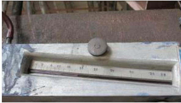
Figure 2.25: Pressure gauge to measure air flow rate
