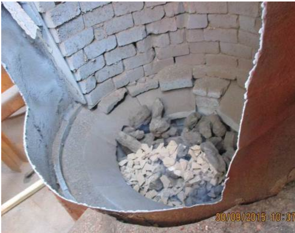
Figure 2.14: Charge loaded from the top during cupola operation
