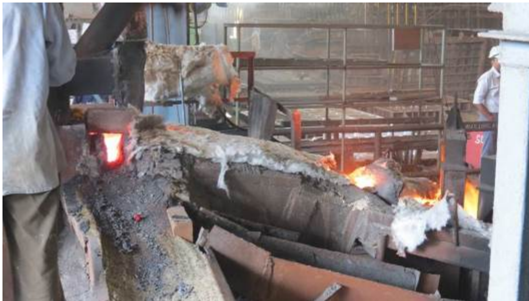
Figure 2.10: Flow of molten metal from cupola
