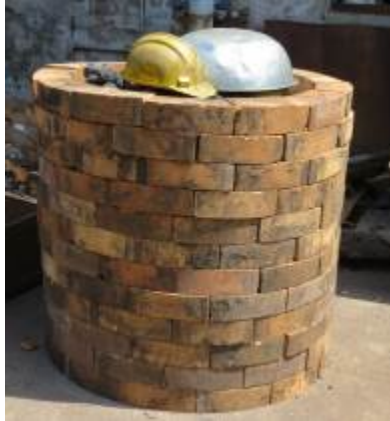
Figure 2.27: Coke bulk density measurement
