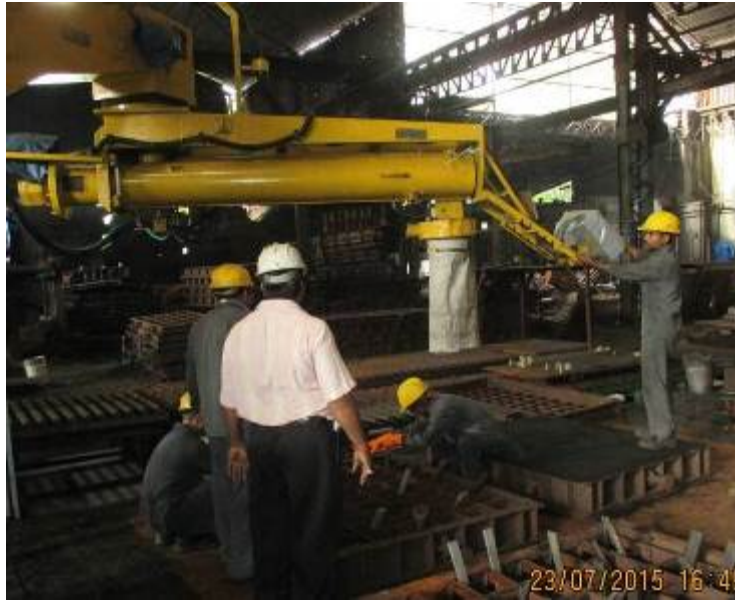
Figure 2.4: Moulding of sands in the pattern
