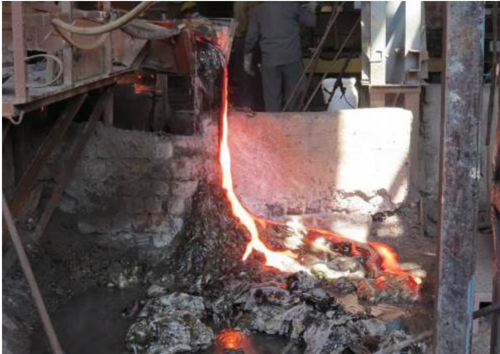
Figure 2.13: Scrap material flowing out of cupola
