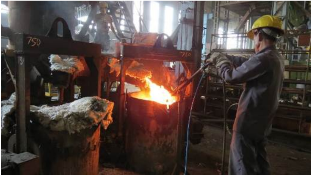
Figure 2.11: Preheating of ladle to avoid any cooling of molten metal
