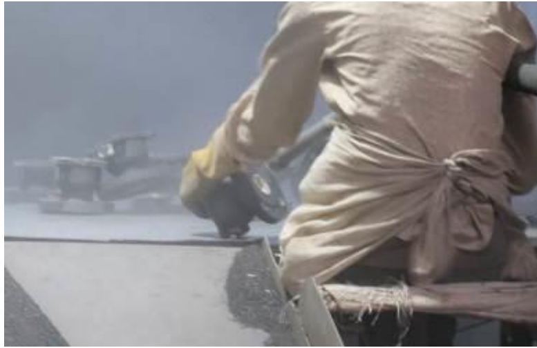
Figure 2.18: Sand blasting for removal of residue of ceramics from final products
