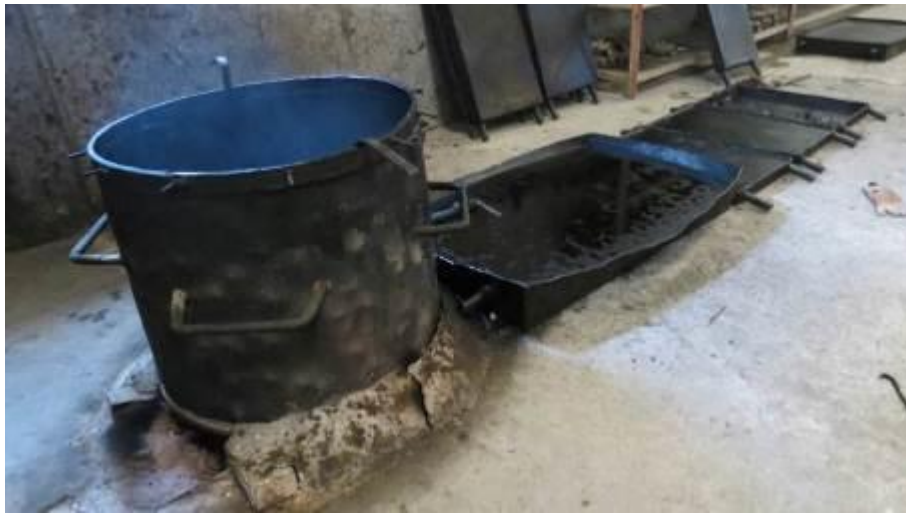
Figure 2.8: Oil fired tank for dewaxing from sand coated moulds
