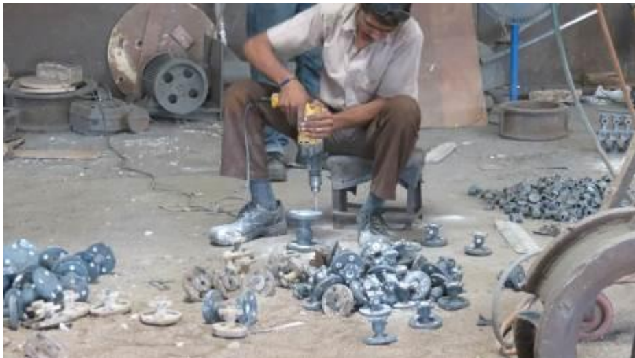
Figure 2.16: Removal of ceramics from holes
