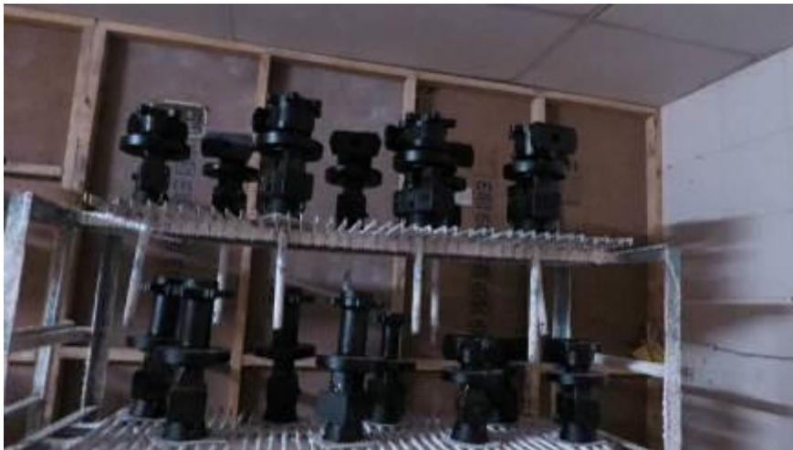
Figure 2.5: Wax pattern after assembly
