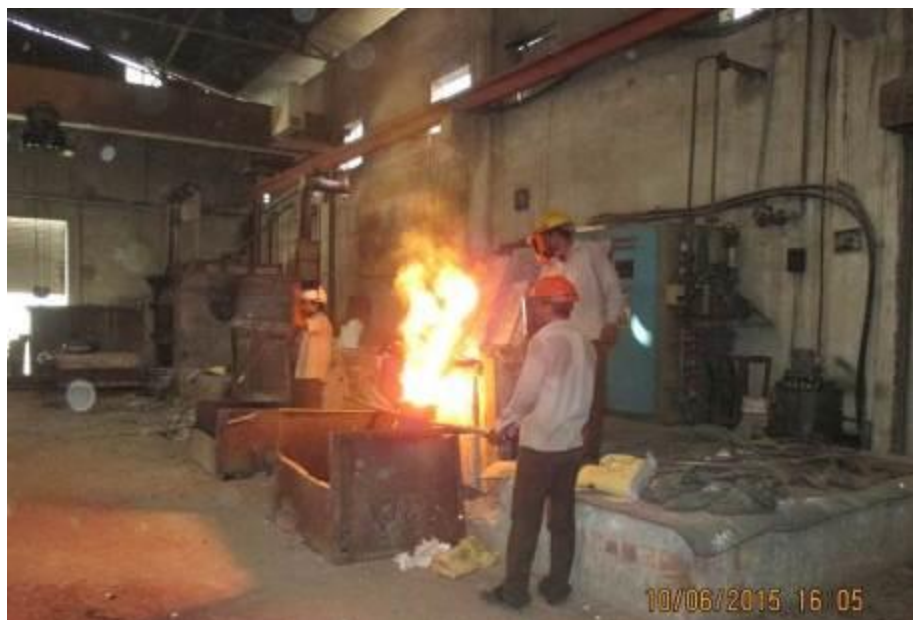
Figure 2.11: Pouring of molten material from crucible to Ladle
