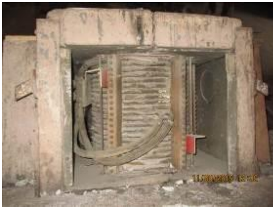
Figure 2.28: Coils of induction furnace around the crucible
