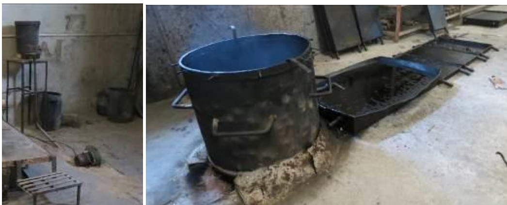
Figure 2.33: Prevailing dewaxing arrangement
