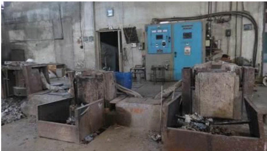
Figure 2.25: Induction furnace along with crucibles
