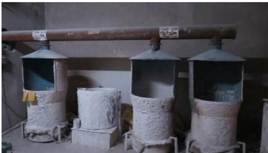
Figure 2.6: Stirrer tank containing ceramic slurry and sand coating equipment
