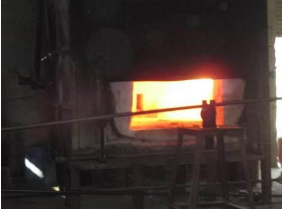
Figure 2.12: Preheating of sand coated moulds in oil fired preheated furnace
