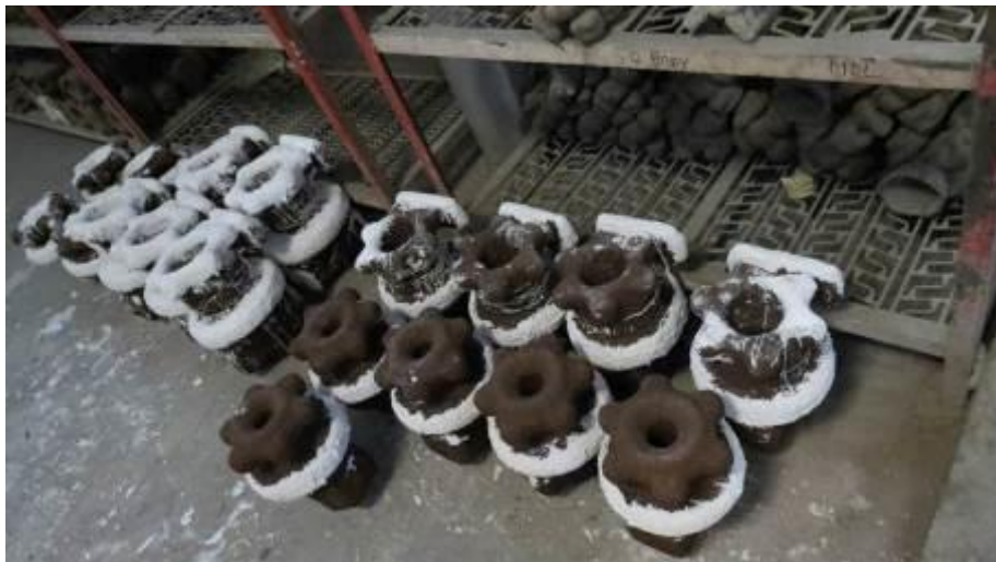
Figure 2.9: Sand coated moulds after dewaxing
