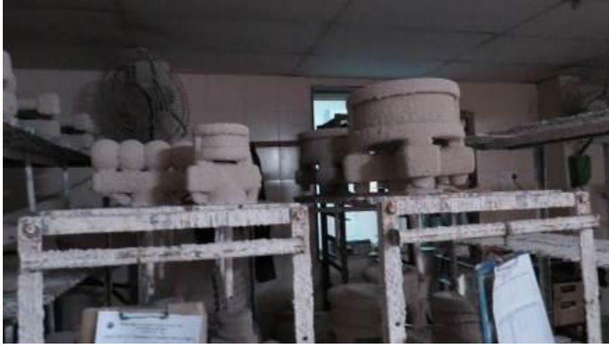
Figure 2.7: Drying of patterns after sand coating
