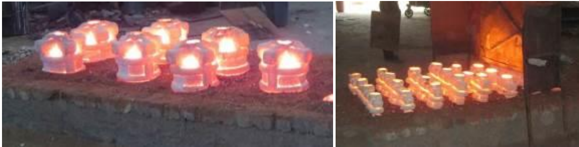
Figure 2.13: Sand coated moulds just after molten metal pouring
