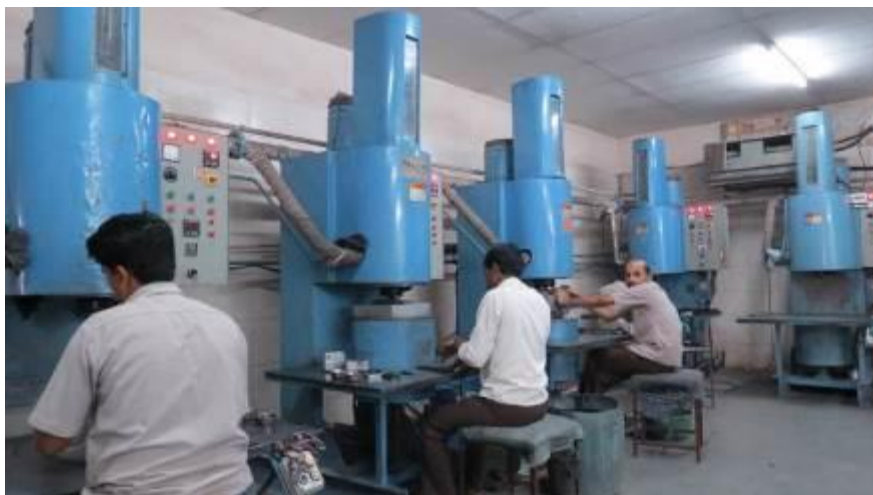
Figure 2.3: Wax pattern making using pneumatic cylinder press
