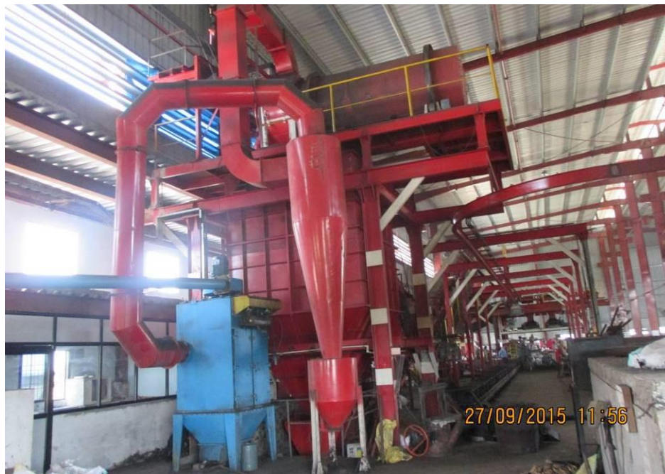
Figure 2.13: Sand mixture and dust separator
