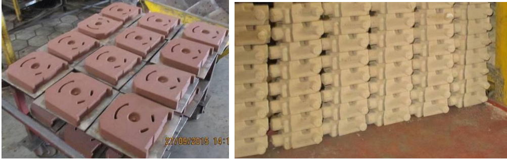
Figure 2.4: Sand cores of different shapes being manufactured
