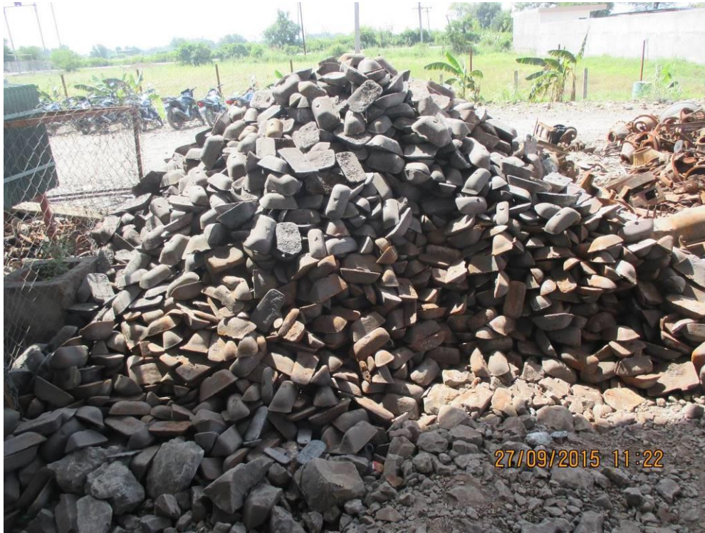
Figure 2.2: Scrap material to be used for melting in Induction furnace
