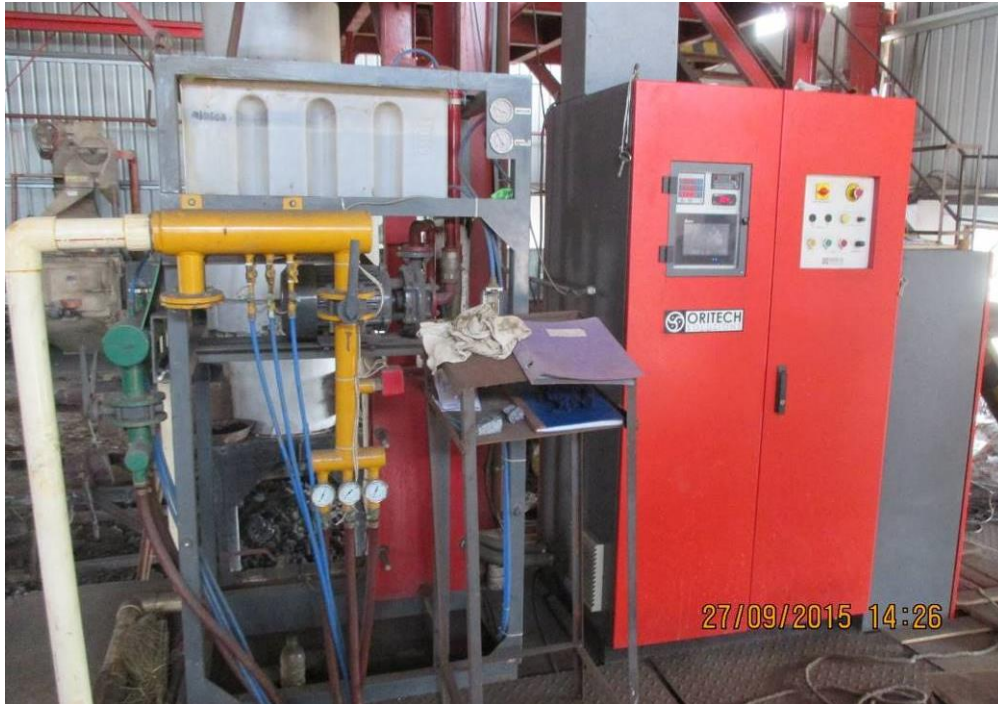
Figure 2.20: Induction furnace along with crucibles installed
