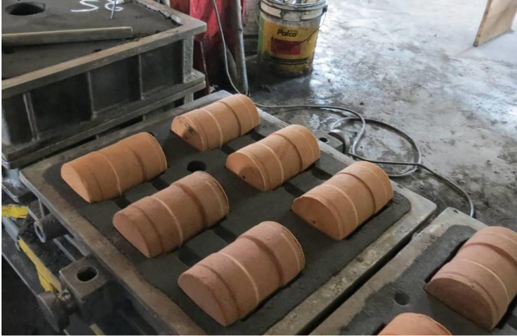
Figure 2.10: Sand cores being placed in moulds
