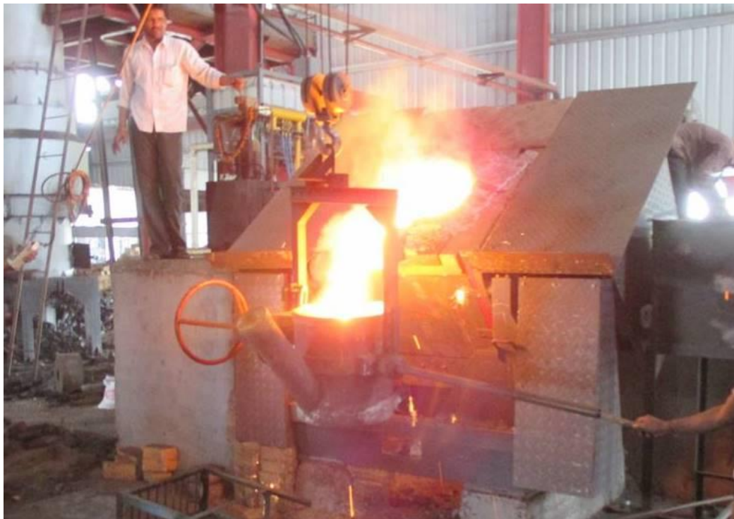
Figure 2.7: Pouring of molten metal from Induction furnace to the Ladle
