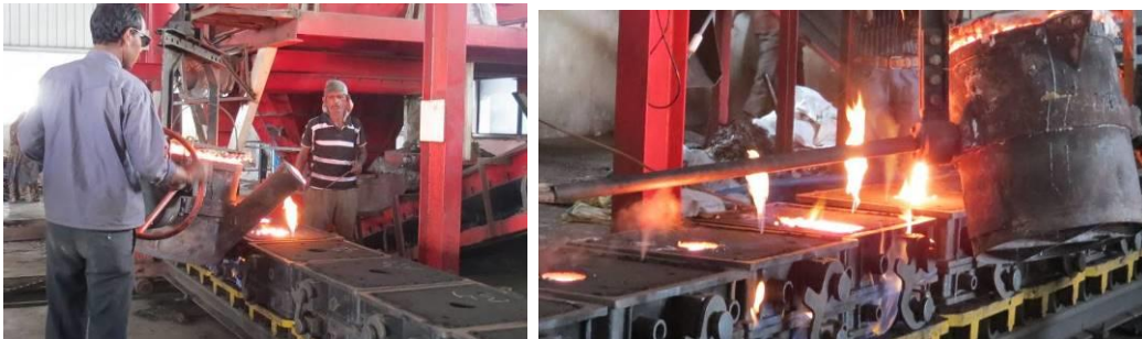
Figure 2.11: Pouring of molten metal from ladle to mould
