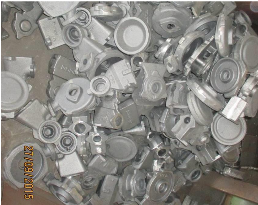
Figure 2.15: Products after shot blast operation
