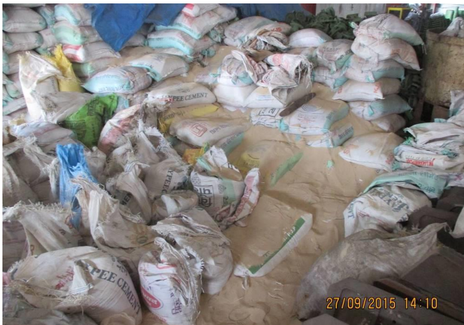
Figure 2.3: Silica sand being used for moulding and core making process
