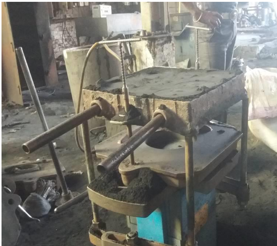
Figure 2.7: Sand mulling for preparation of mould
