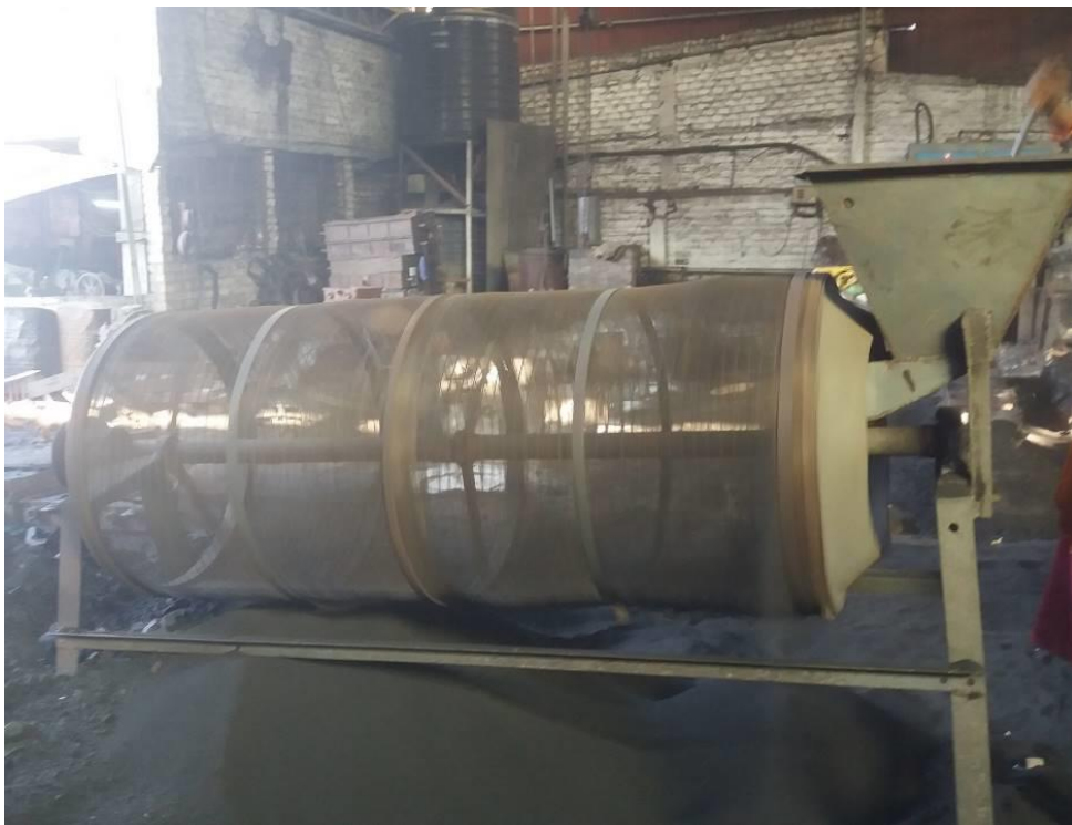
Figure 2.5: Sand sieve for sieving the recycled sand
