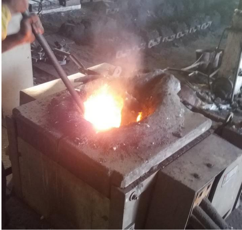
Figure 2.12: Poking of material in the furnace
