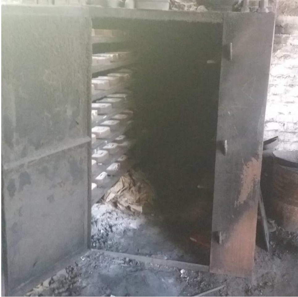
Figure 2.4: Closed furnace for baking of sand cores
