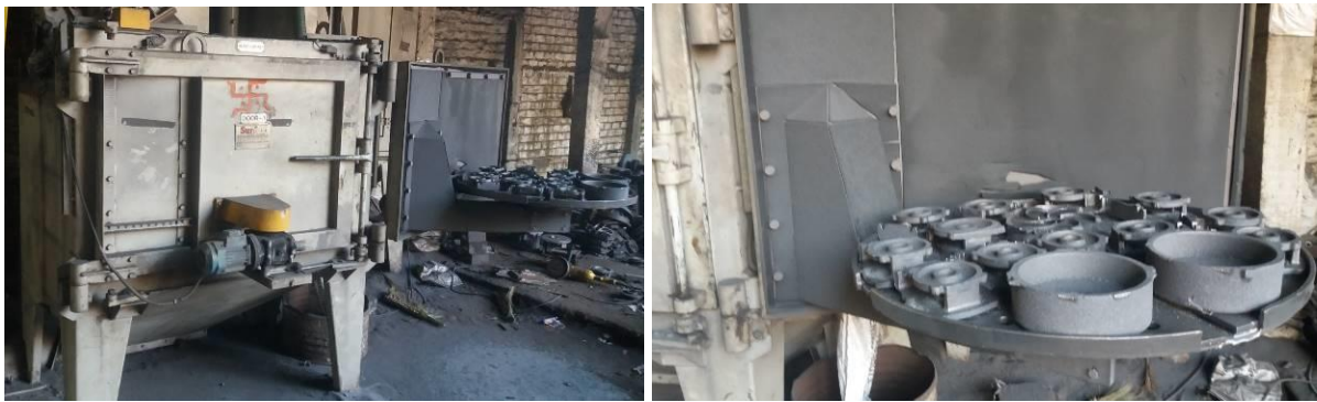
Figure 2.17: Shot blast machine and casting ready for shot blast for operation
