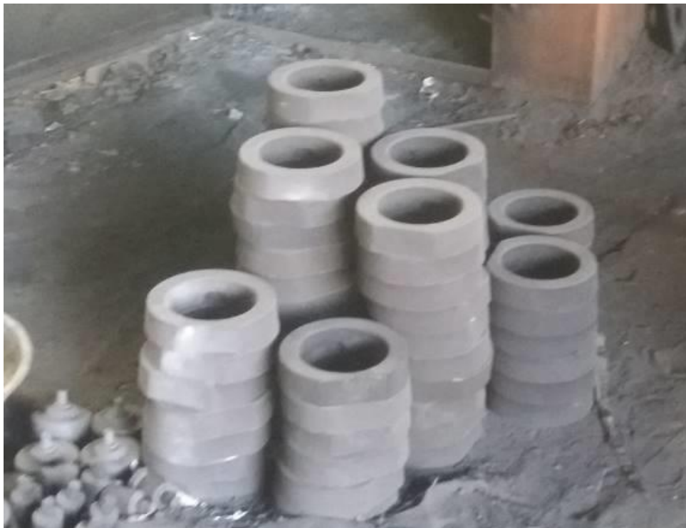
Figure 2.3: Sand core prepared through oil core process
