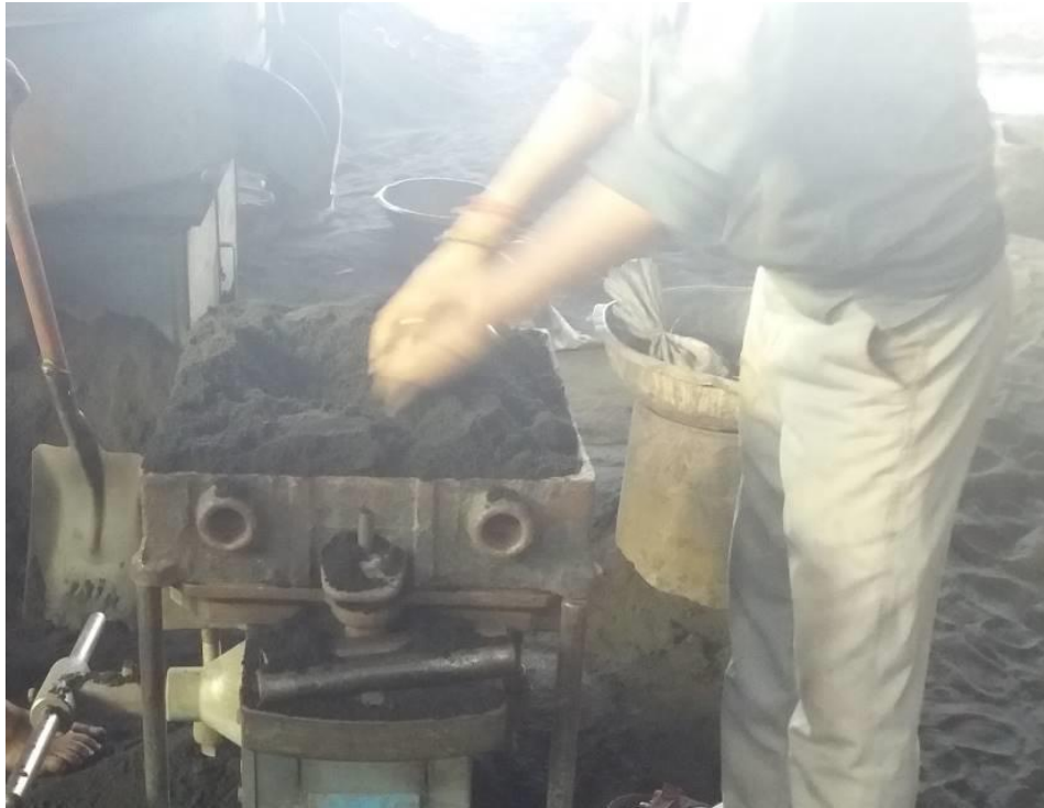
Figure 2.8: Filling of moulding sand in pattern for preparation of mould
