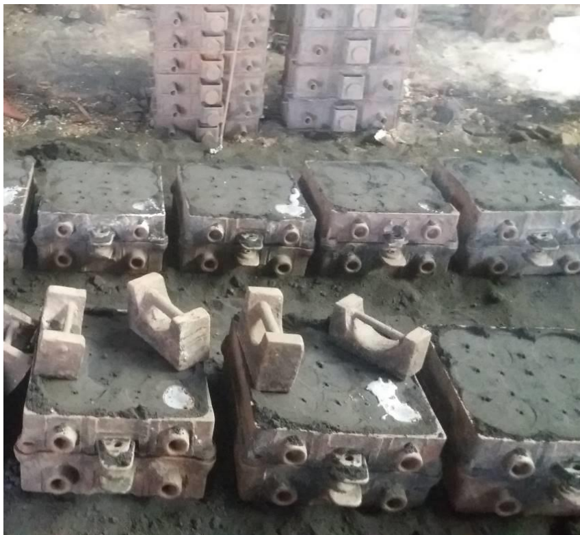
Figure 2.15: Moulds left for cooling after pouring
