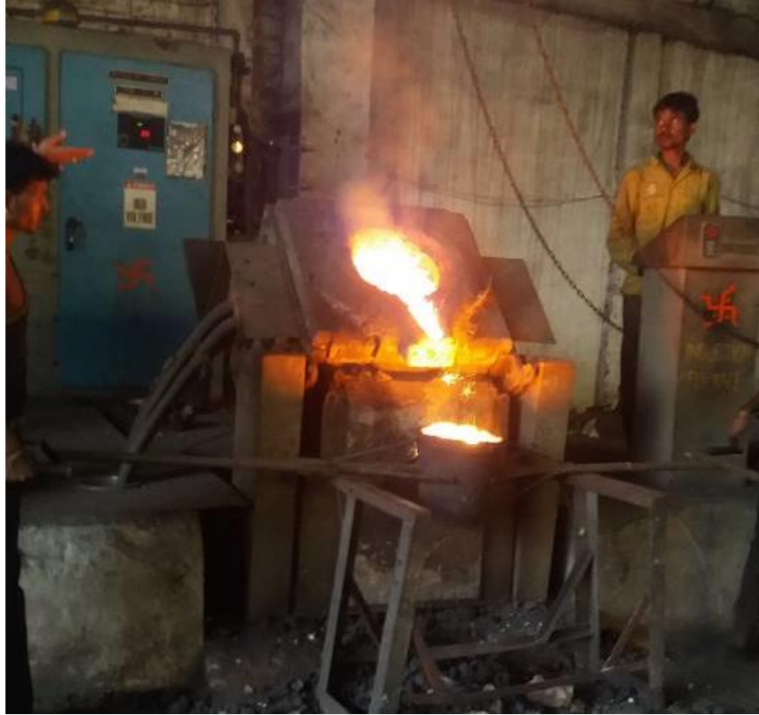
Figure 2.14: Pouring of metal from furnace to ladle
