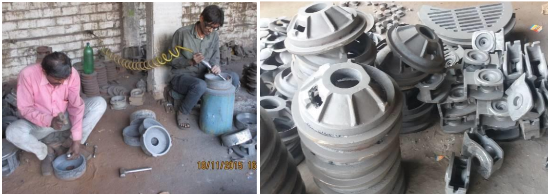
Figure 2.18: Grinding of castings and finished products
