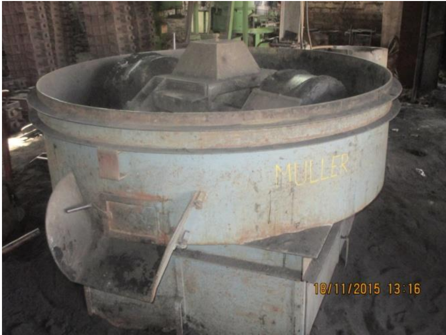
Figure 2.6: Sand muller for preparation of moulding sand
