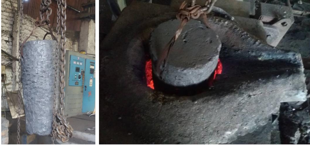
Figure 2.25: Graphite piece placed inside the crucible
