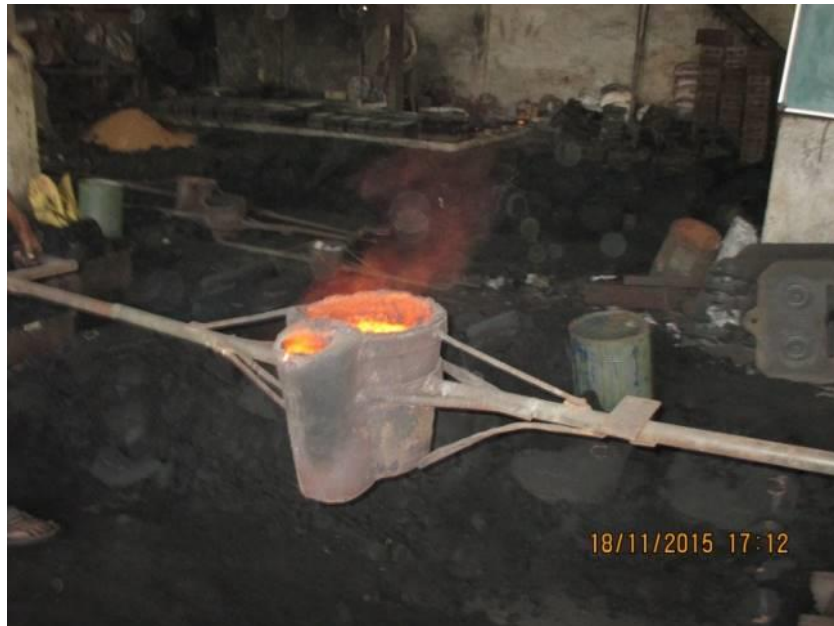
Figure 2.13: Ladle for pouring of molten metal
