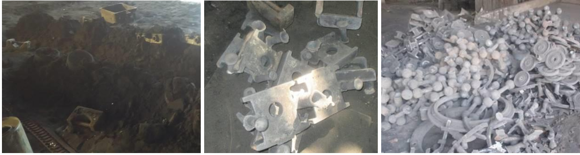
Figure 2.16: Castings after knockout
