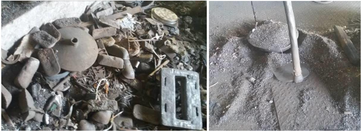
Figure 2.10: Raw material being used in the induction furnace
