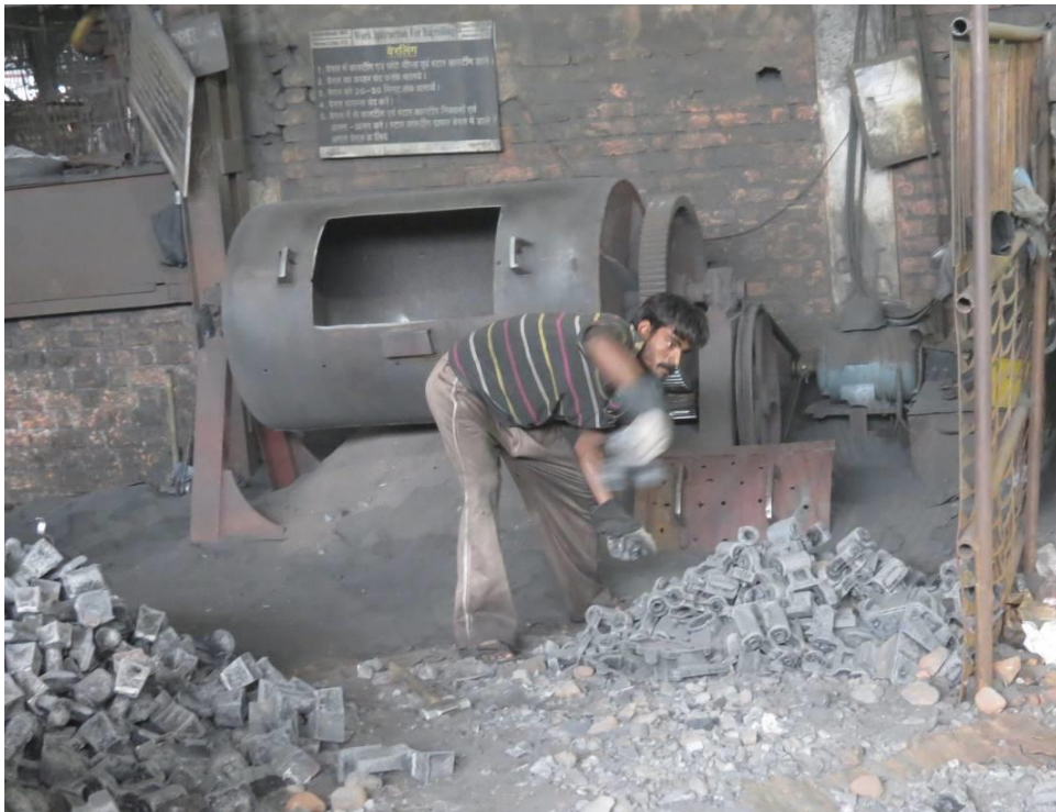
Figure 2.14: Removal of residual sand from castings
