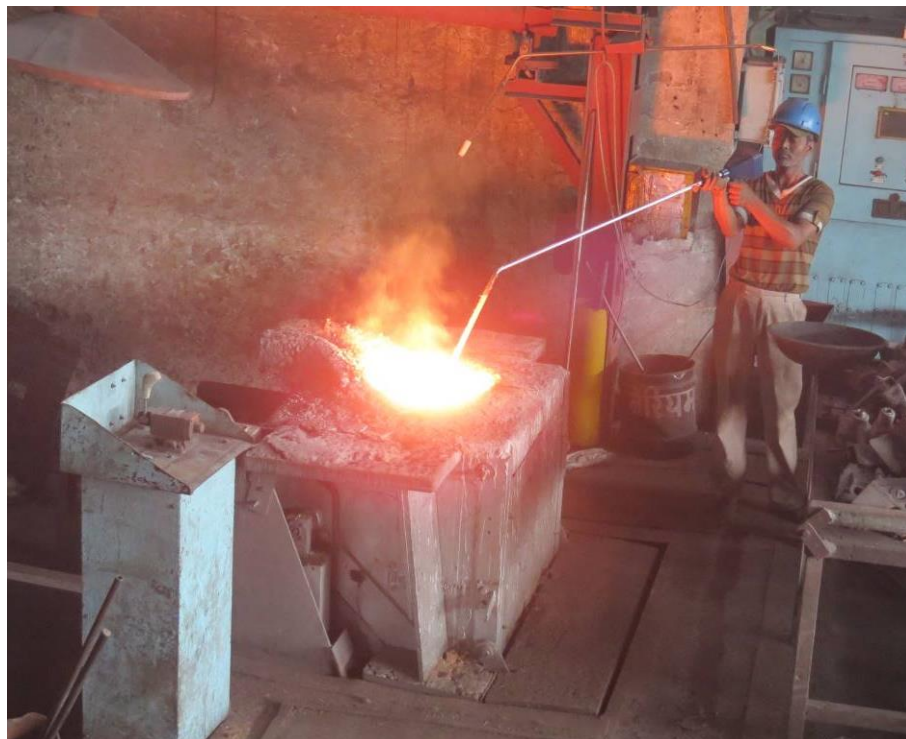
Figure 2.10: Measurement of temperature of molten material
