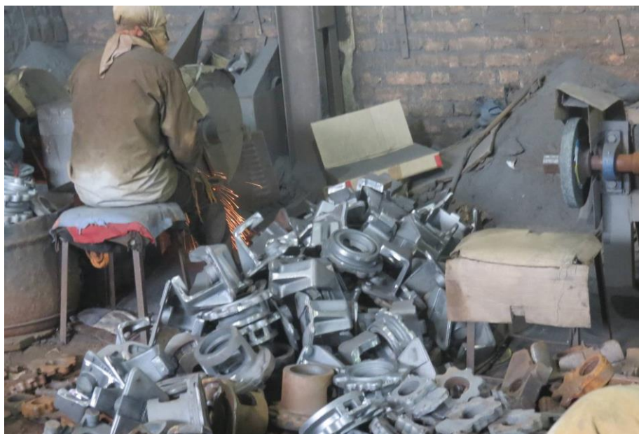
Figure 2.17: Grinding of castings to improve surface finish
