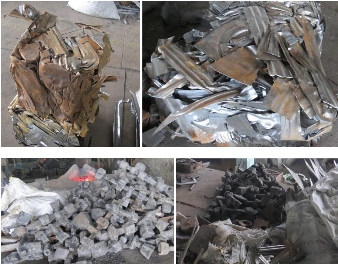
Figure 2.8: Raw material to be used in Induction furnace
