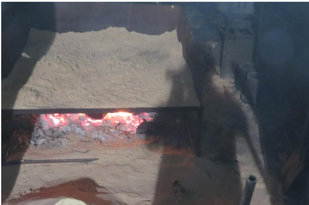
Figure 2.3: Drying of sand using wood based burning
