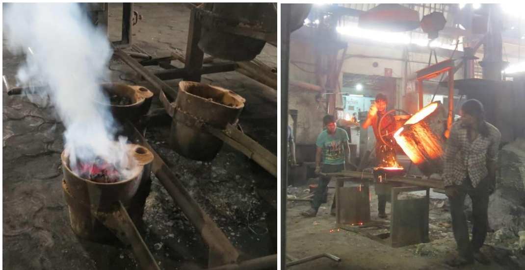
Figure 2.12: Preheating of ladle and pouring of molten material into ladle
