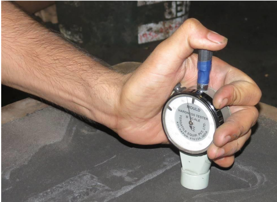
Figure 2.7: Hardness testing of moulds
