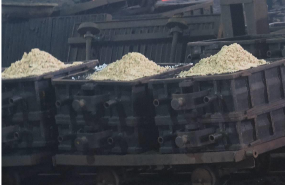
Figure 2.13: Moulds after pouring
