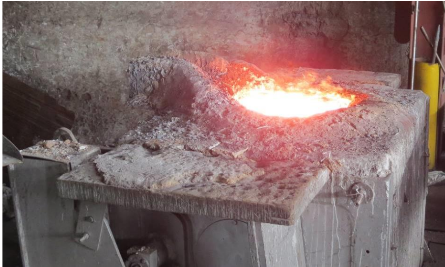
Figure 2.9: Melting of scrap material in Induction furnace
