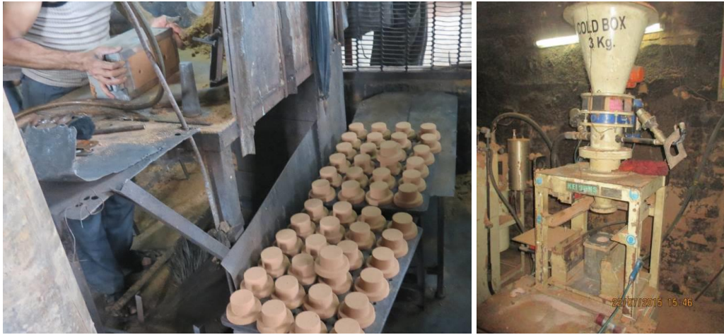
Figure 2.4: Cold box machine and cores prepared
