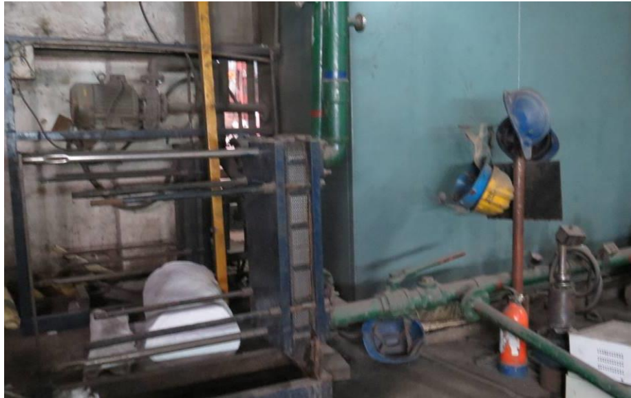
Figure 2.11: Heat exchanger for removal of furnace heat
