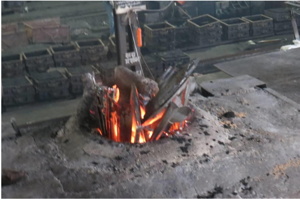
Figure 2.22: Filling of scrap material in the induction furnace
