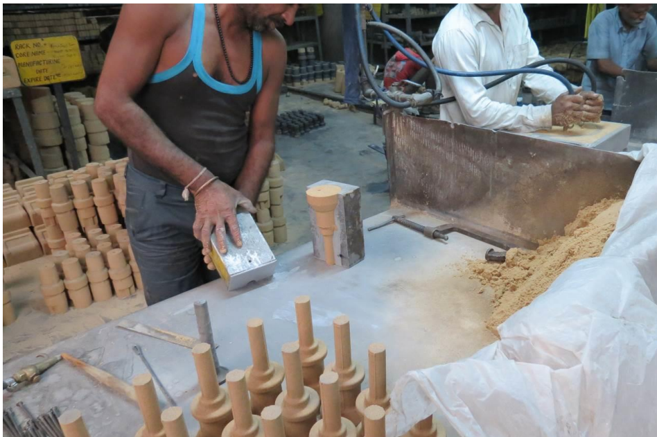
Figure 2.5: Core making in progress
