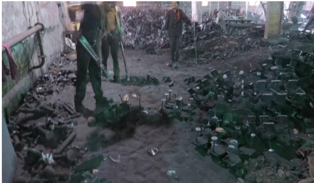
Figure 2.15: Manual de-coring of castings
