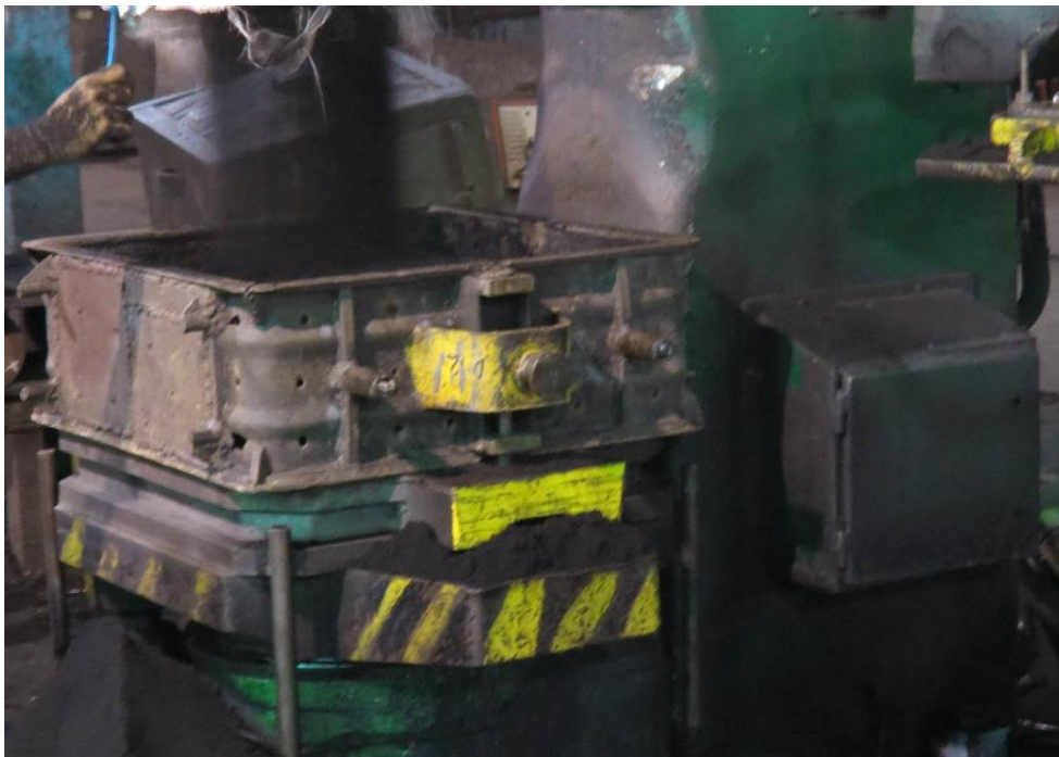
Figure 2.11: Sand moulding in progress
