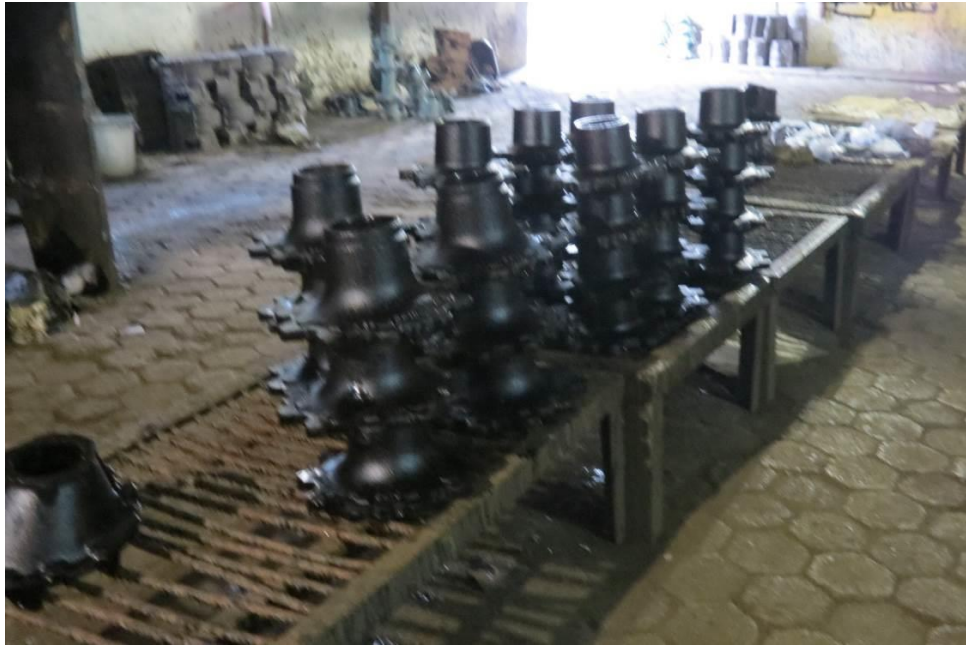
Figure 2.20: Final casting after painting
