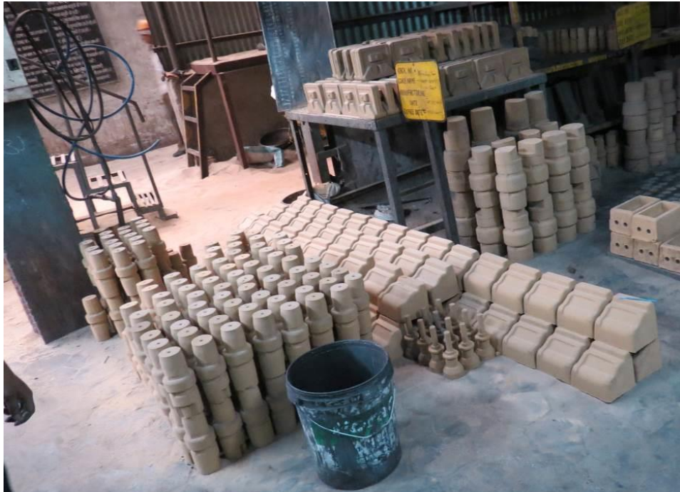
Figure 2.6: Sand cores of different shapes being manufactured
