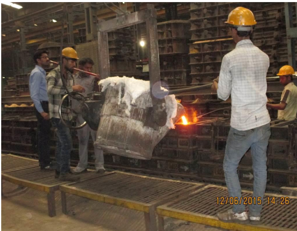
Figure 2.13: Pouring of molten metal
