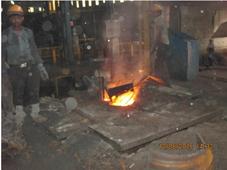
Figure 2.8: Melting of scrap material in the furnace
