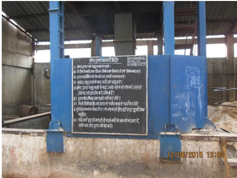
Figure 2.3: Sand dryer for reducing moisture content of the sand
