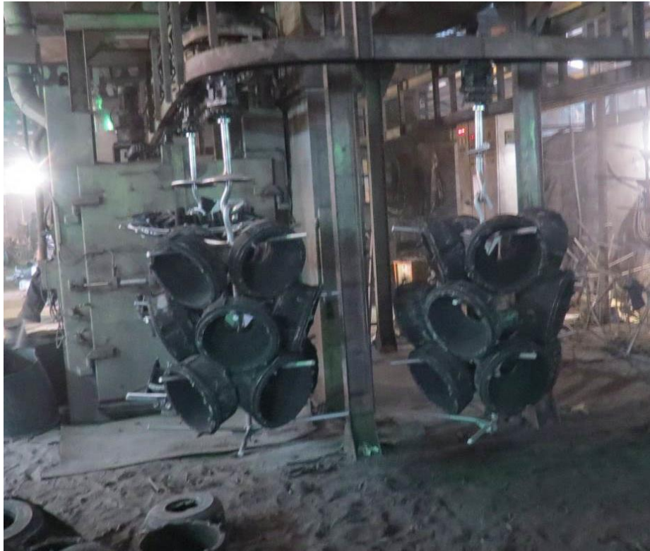
Figure 2.16: Casting before sand blasting operation
