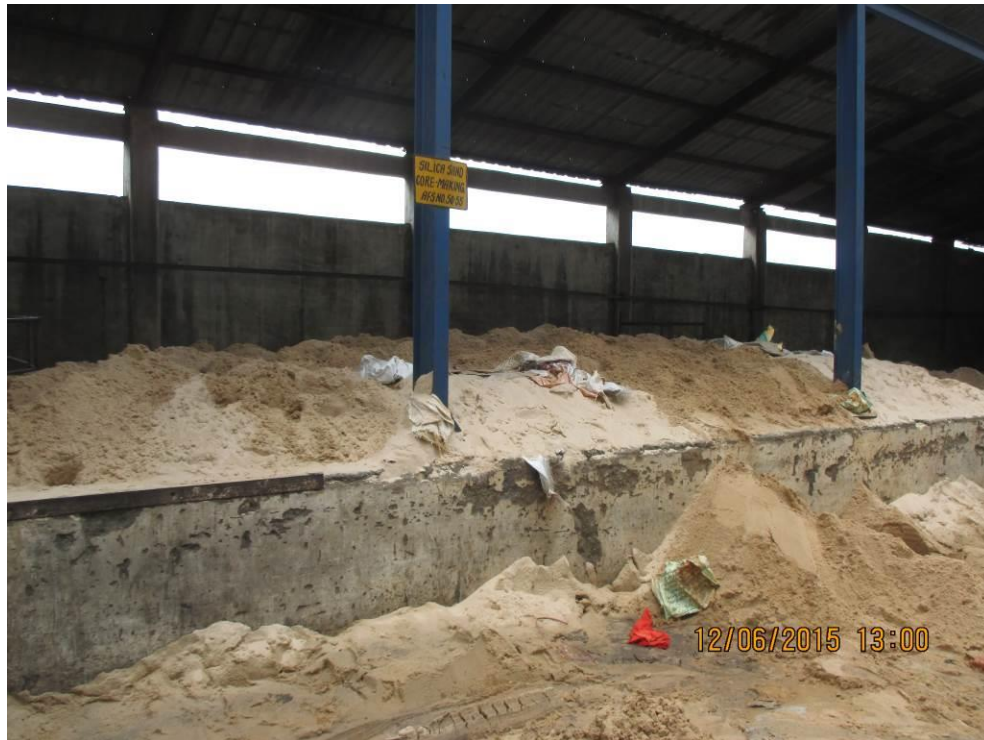
Figure 2.2: Silica sand being used for moulding and core making process
