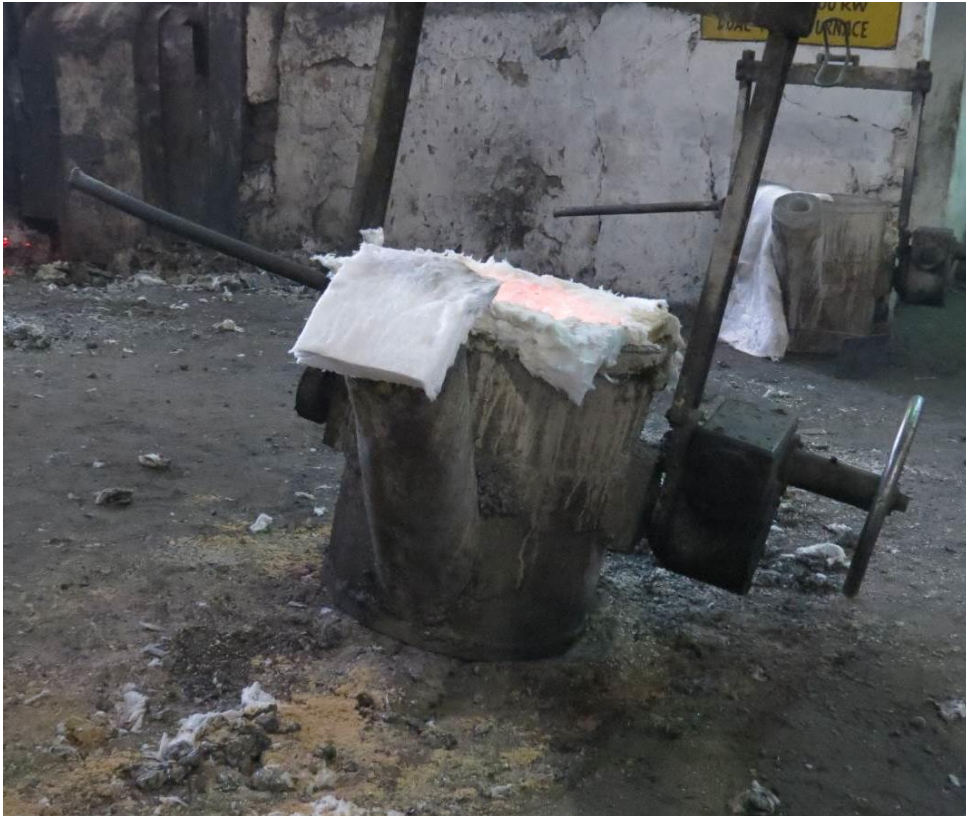
Figure 2.10: Ladle containing molten metal
