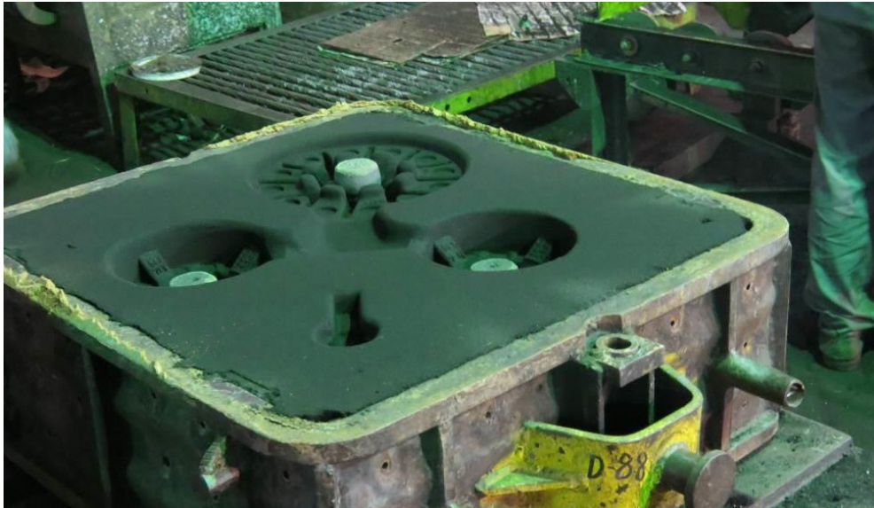
Figure 2.12: Half Sand mould containing required cavity
