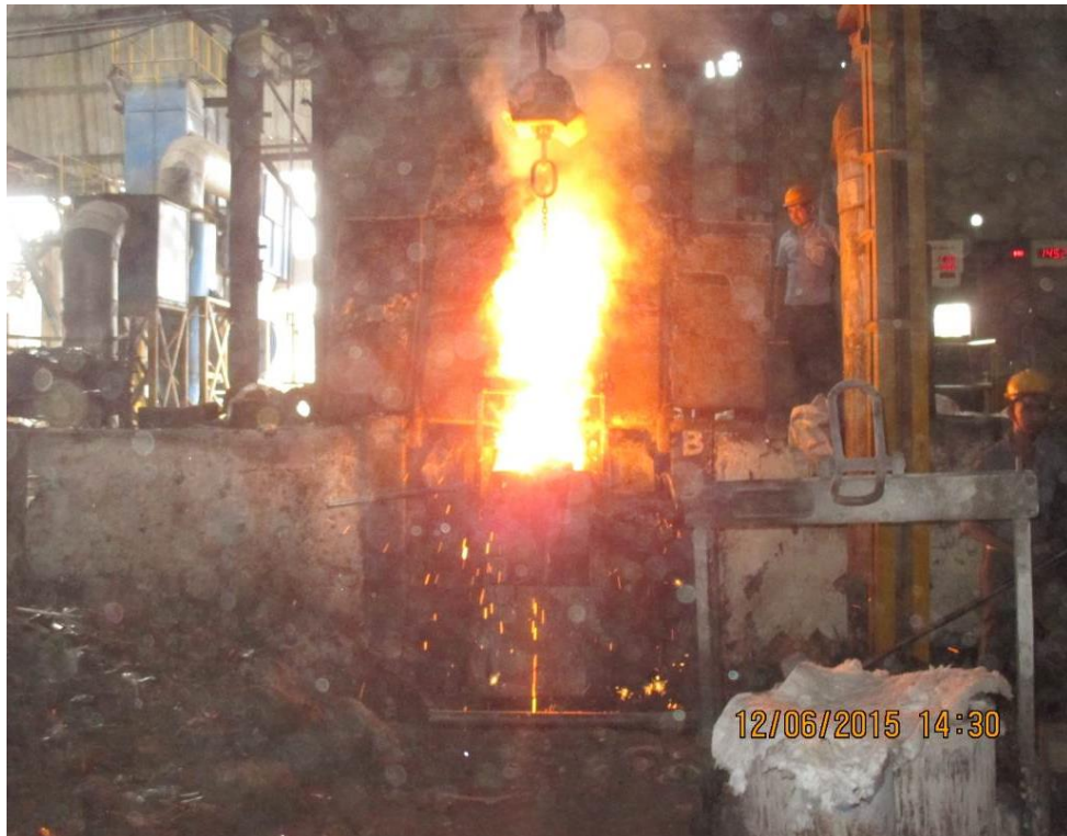
Figure 2.9: Transfer of molten metal from furnace to ladle
