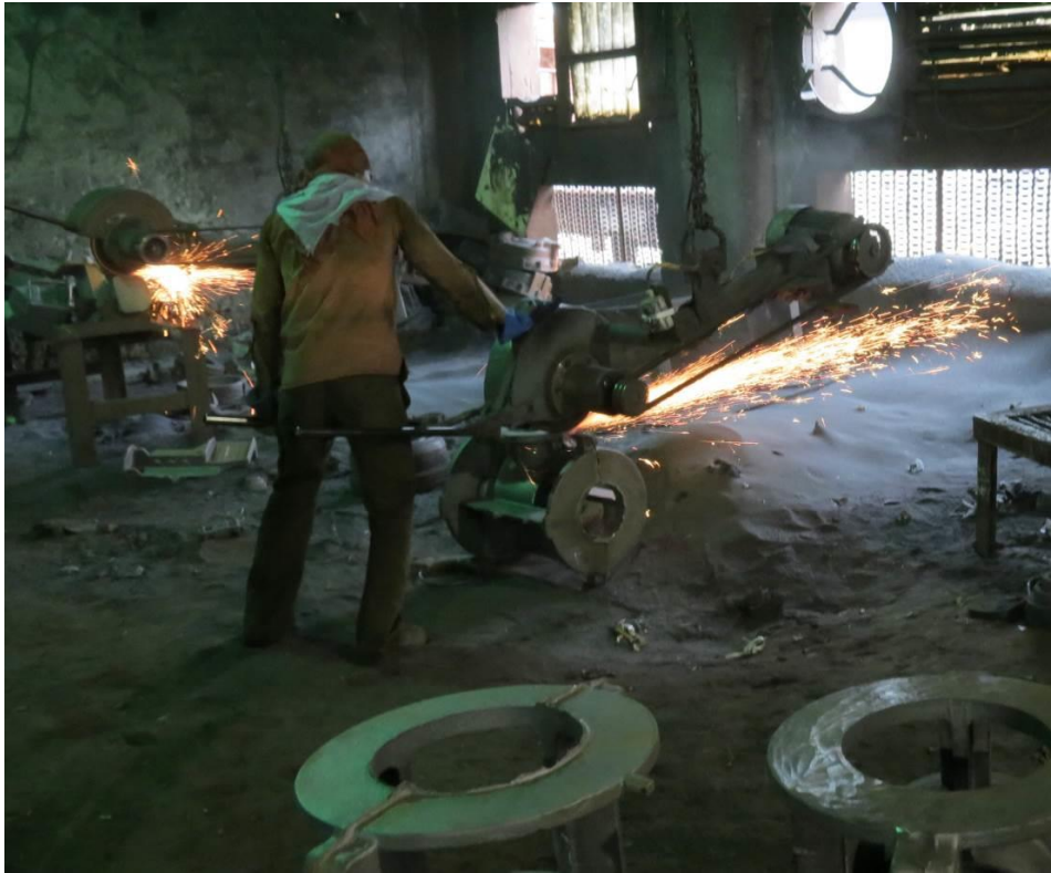
Figure 2.18: Grinding of the casting
