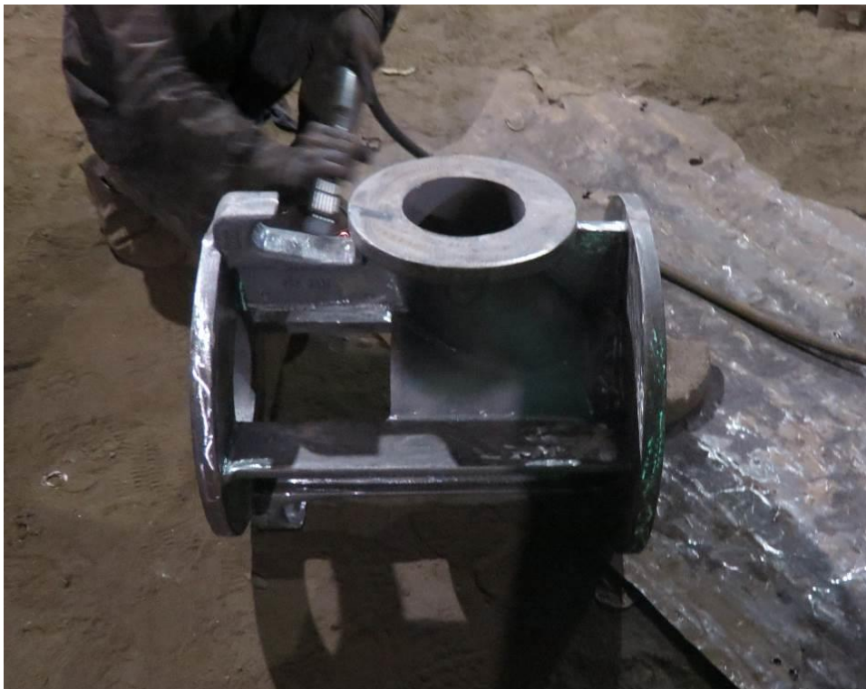
Figure 2.19: Grinding of casting using pneumatic tool
