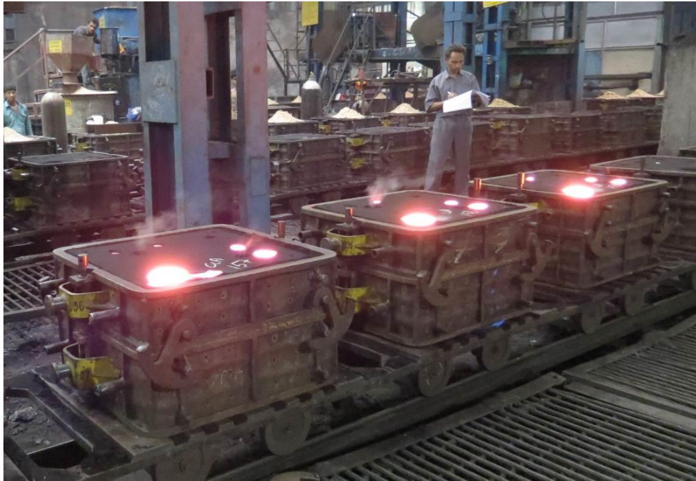
Figure 2.14: Sand moulds after metal pouring
