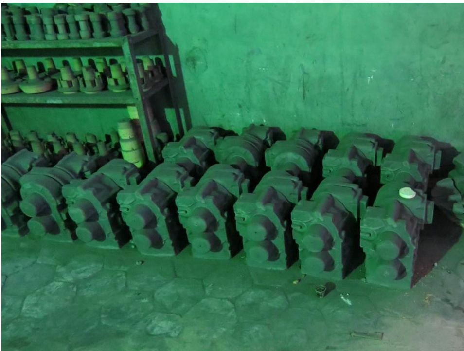
Figure 2.7: Final sand cores after performing finishing and painting operations
