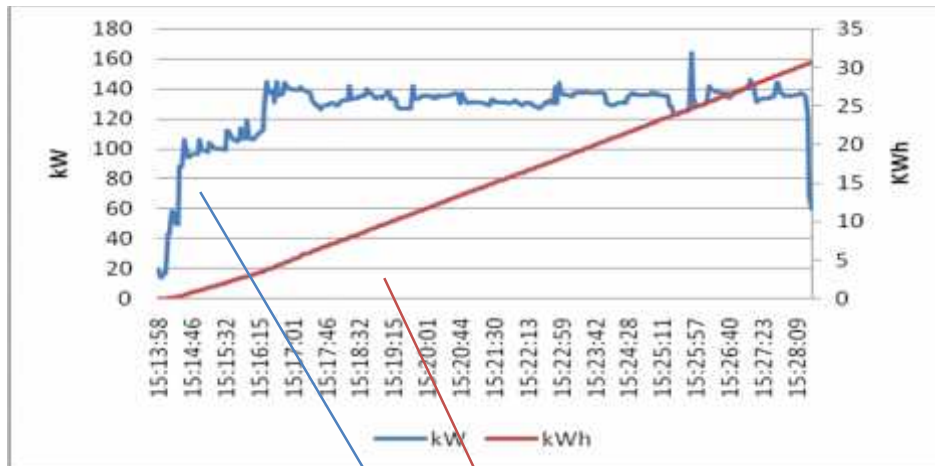
Figure 16: DG – 2 (250 kVA) test graph
