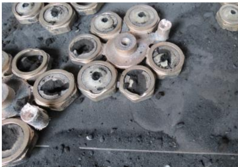
Figure 2.6: Castings after pouring
