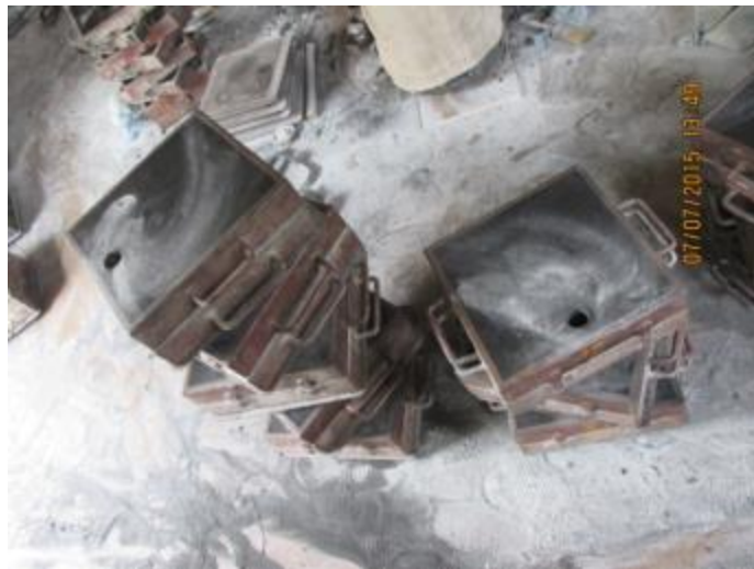
Figure 2.3: Sand moulds ready for pouring
