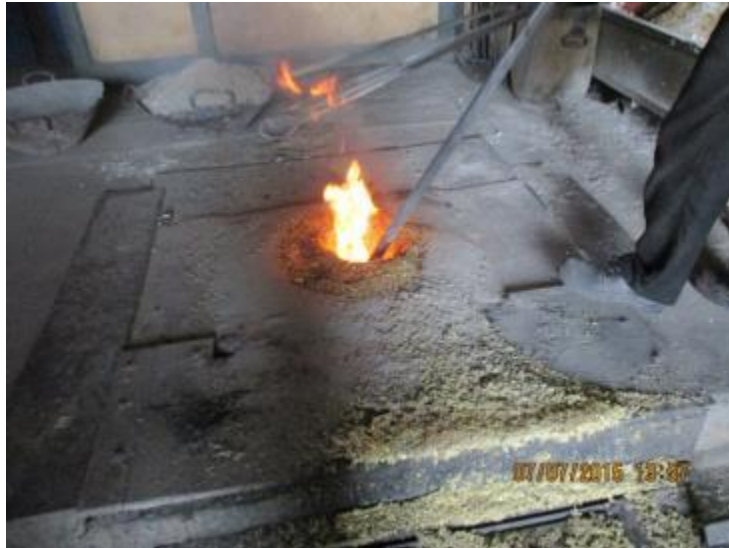
Figure 2.4: Melting of scrap material in Induction furnace
