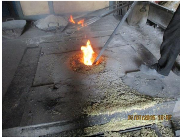
Figure 2.11: Heating of material in induction melting furnace
