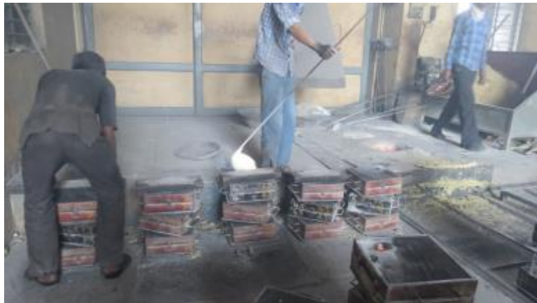
Figure 2.5: Poring of molten material in sand moulds
