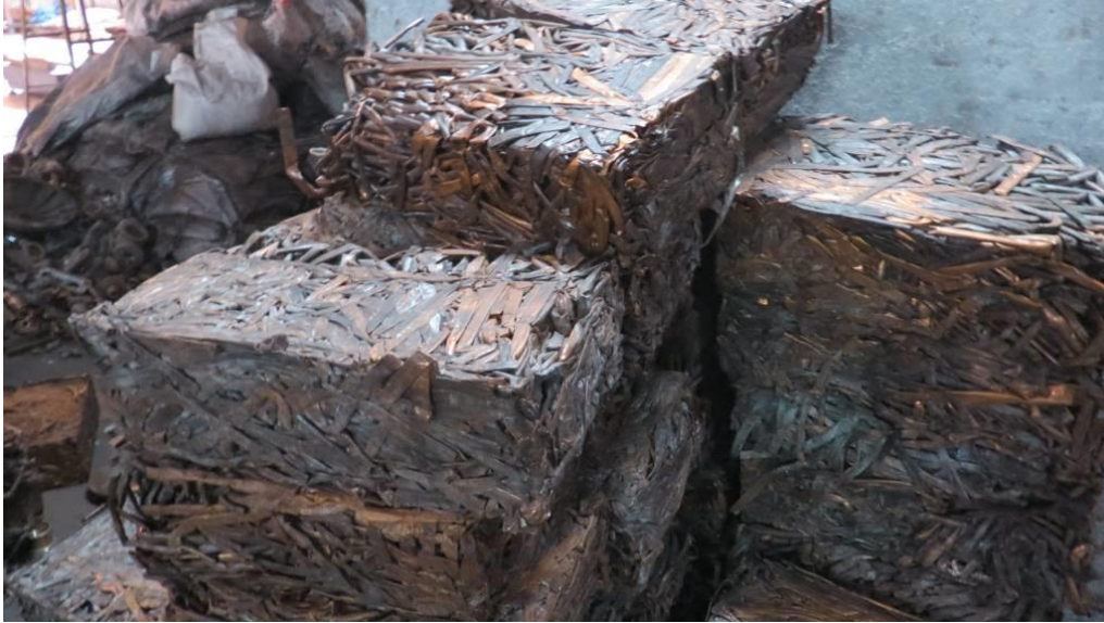
Figure 2.5: Raw material after compaction in the bailing machine
