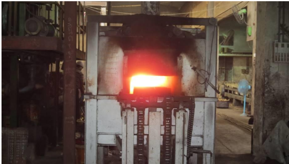
Figure 2.11: Heating of material in reheating furnace
