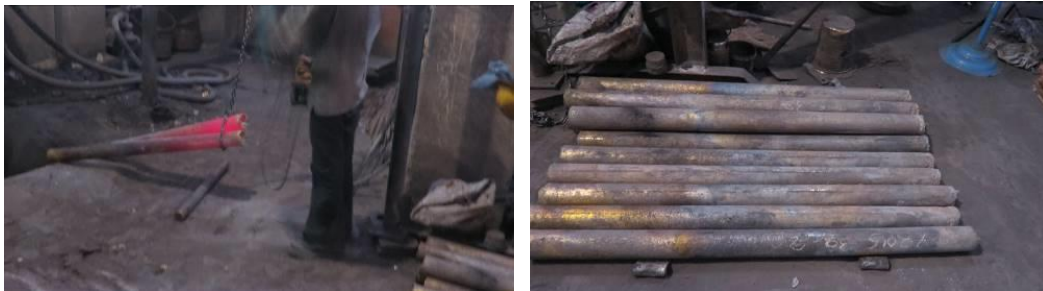
Figure 2.8: Billet prepared from the molten material
