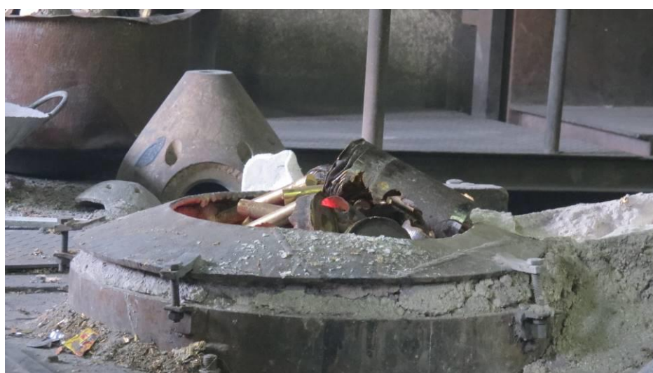
Figure 2.24: Heating of material in reheating furnace
