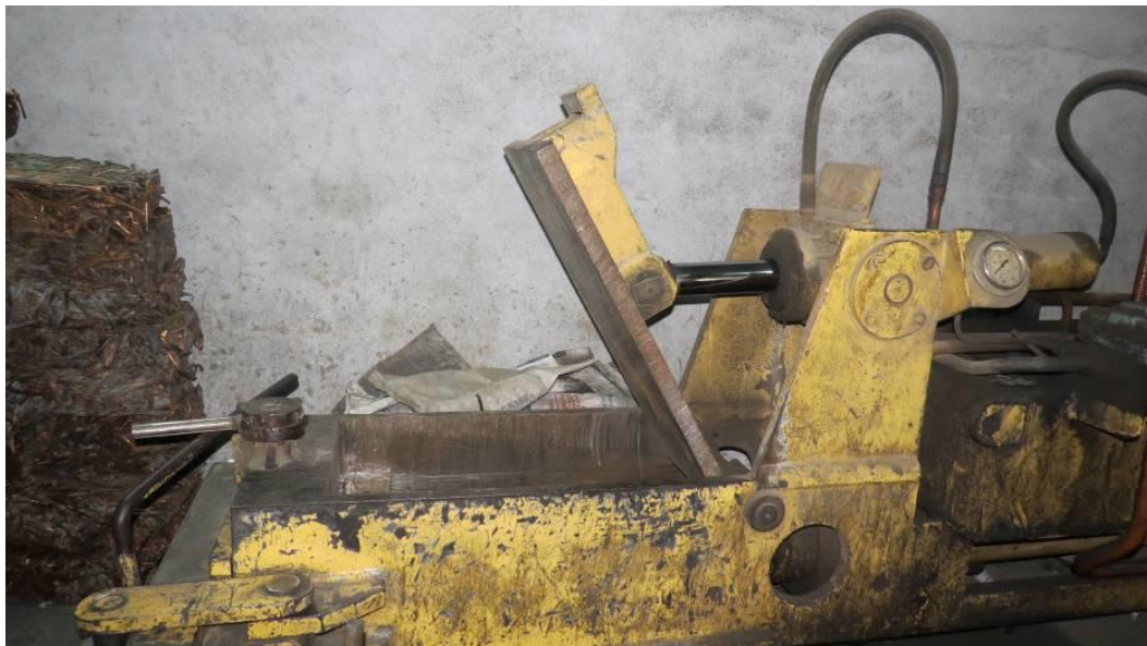
Figure 2.4: Baling machine being used for compaction of selected raw material
