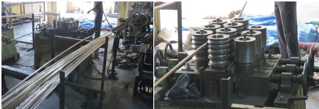
Figure 2.17: Straightening of rods
