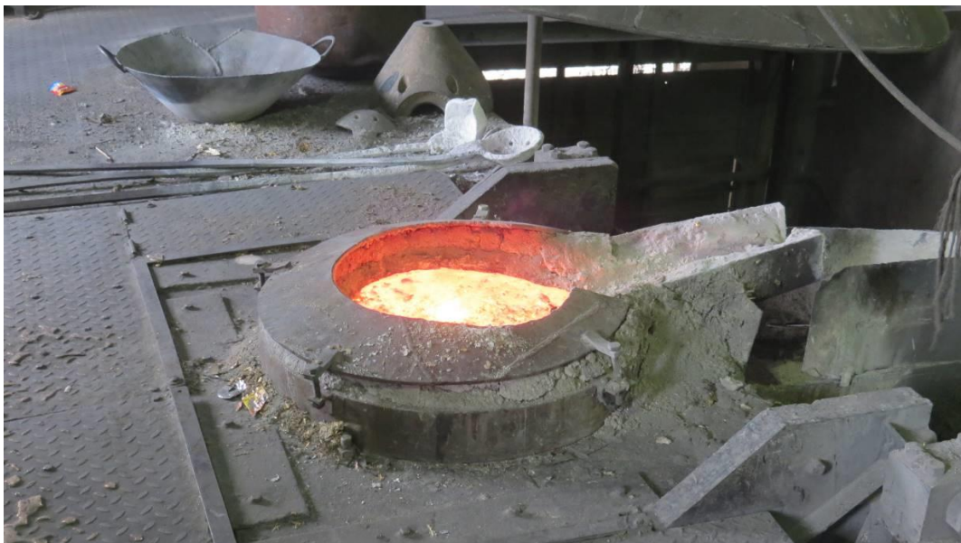
Figure 2.6: Melting of raw material in the induction furnace
