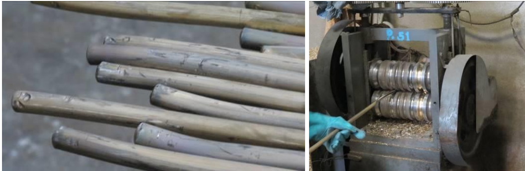
Figure 2.14: Front end of the rod material before pointing and pointing operation in progress
