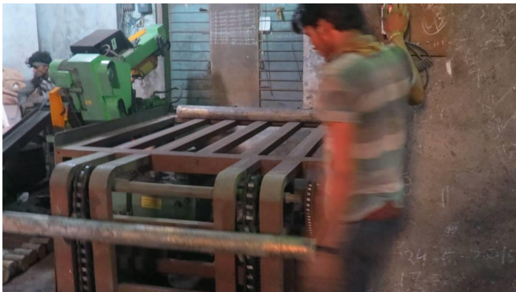
Figure 2.9: Shearing machine for cutting of the billets
