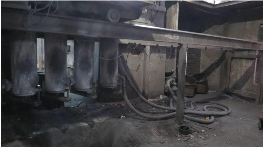
Figure 2.7: Pouring of raw material in cylinders to make billets
