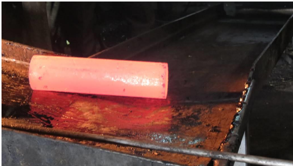
Figure 2.12: Heated material coming out from reheating furnace
