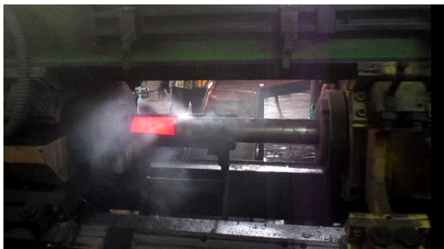
Figure 2.25: Hot drawing in extrusion press
