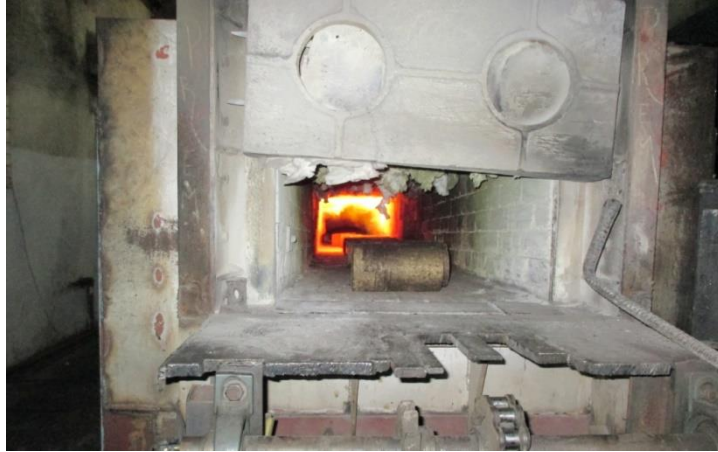
Figure 2.9: Feeding of billet piece into the reheating furnace
