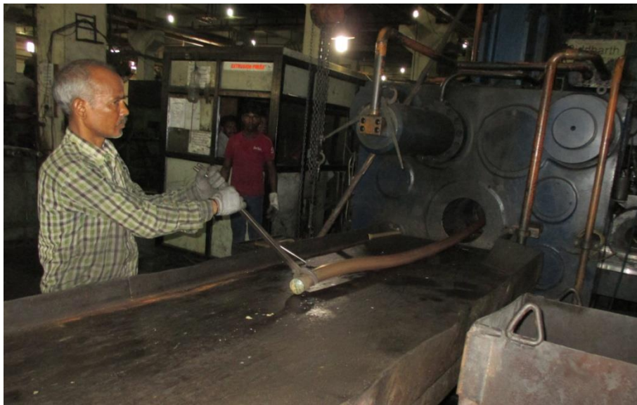
Figure 2.10: Drawing of heated material in extrusion machine
