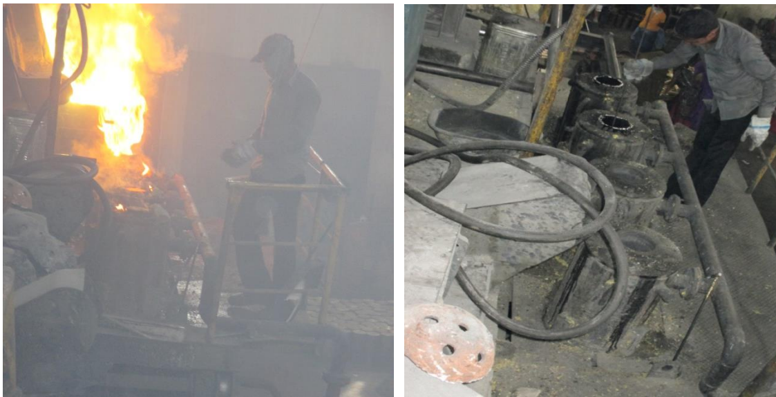
Figure 2.5: Pouring of molten metal
