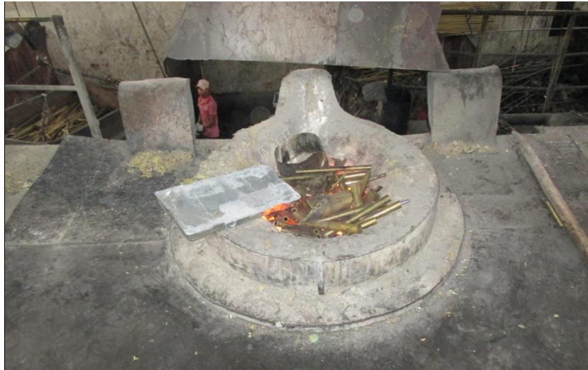
Figure 2.15: Heating of material in induction melting furnace
