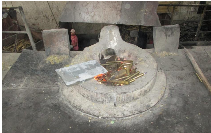
Figure 2.3: Feeding of scrap material in the induction furnace
