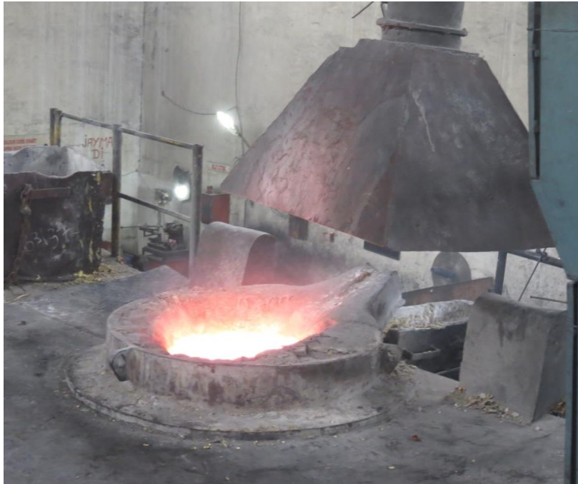
Figure 2.4: Melting of scrap material in the induction furnace
