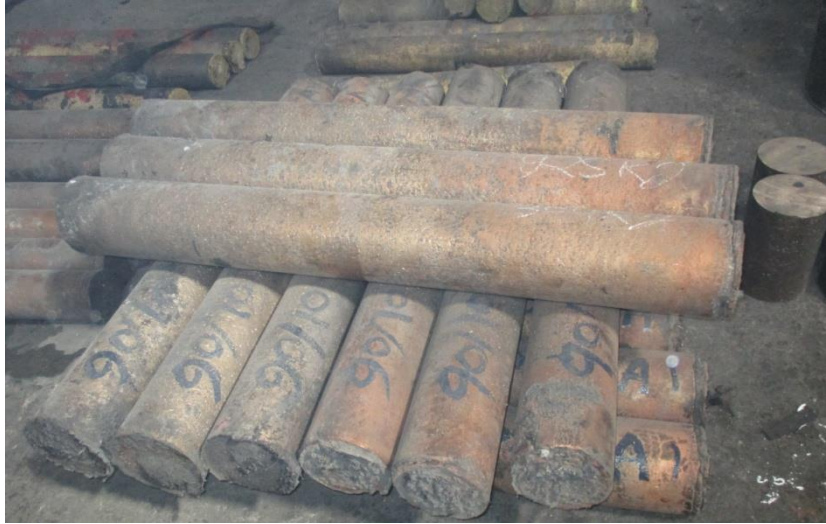
Figure 2.6: Billet produced after cooling
