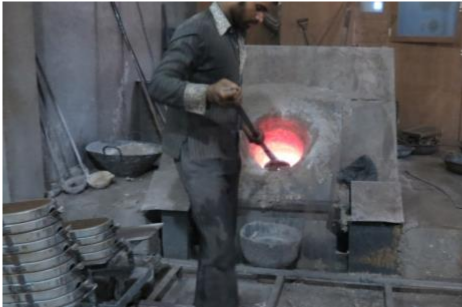
Figure 2.6: Removal of scrap from induction furnace
