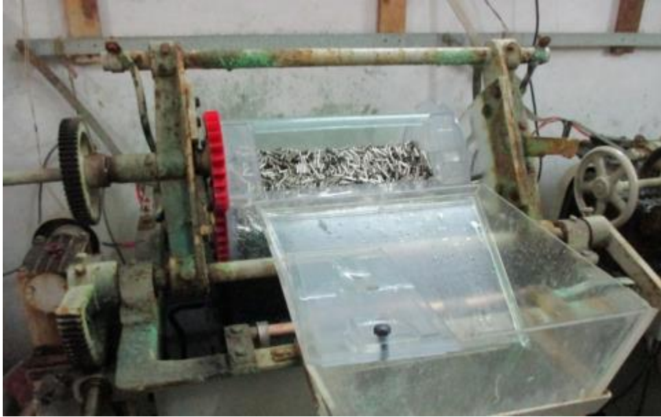
Figure 2.13: Products subjected to electroplating operation
