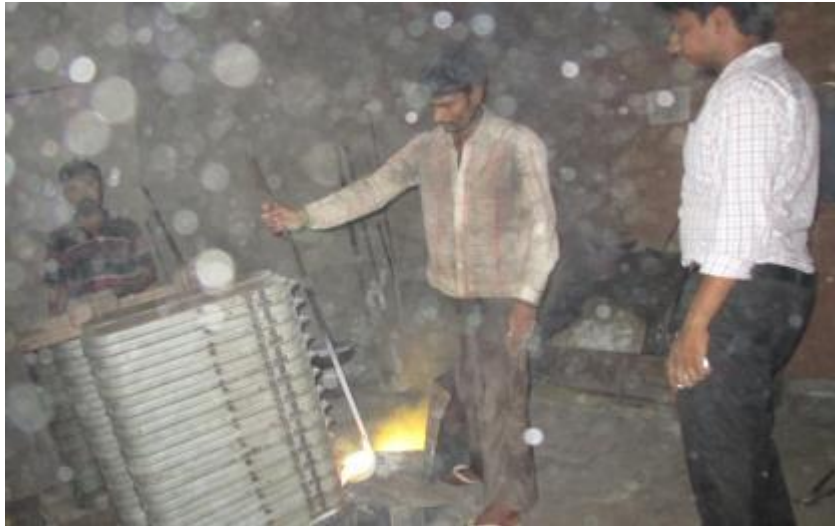
Figure 2.7: Pouring of molten metal into sand moulds
