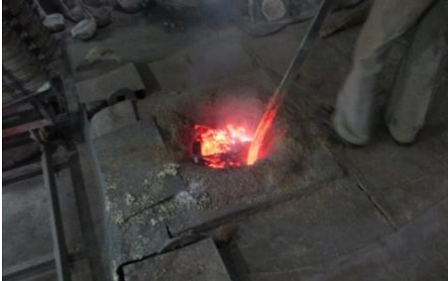
Figure 2.5: Scrap melting in the induction furnace
