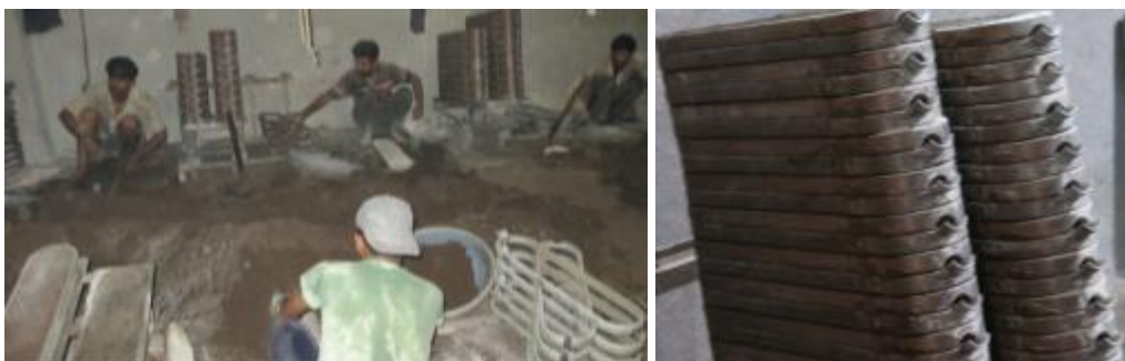
Figure 2.4: Preparation of sand mould
