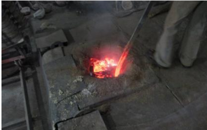
Figure 2.18: Heating of material in induction melting furnace
