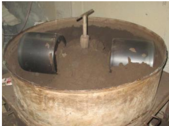
Figure 2.3: Sand Muller for preparation of moulding sand
