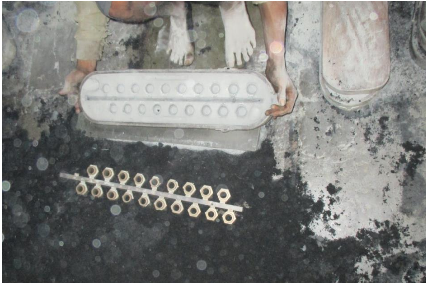
Figure 2.4: Preparation of sand mould
