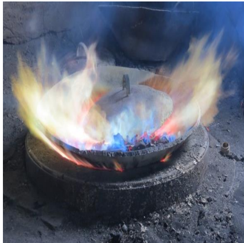
Figure 2.11a: Actual coke pit furnace
