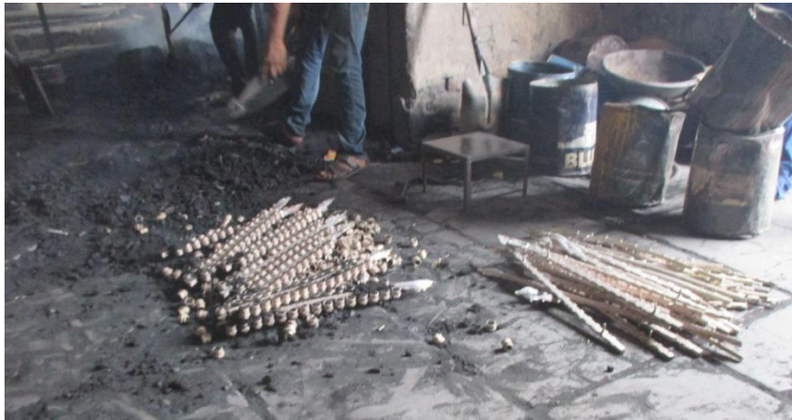
Figure 2.7: Separation of sand and casting in the knockout section
