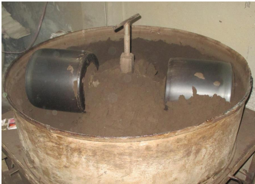
Figure 2.3: Sand Muller machine for mixing of moulding sand
