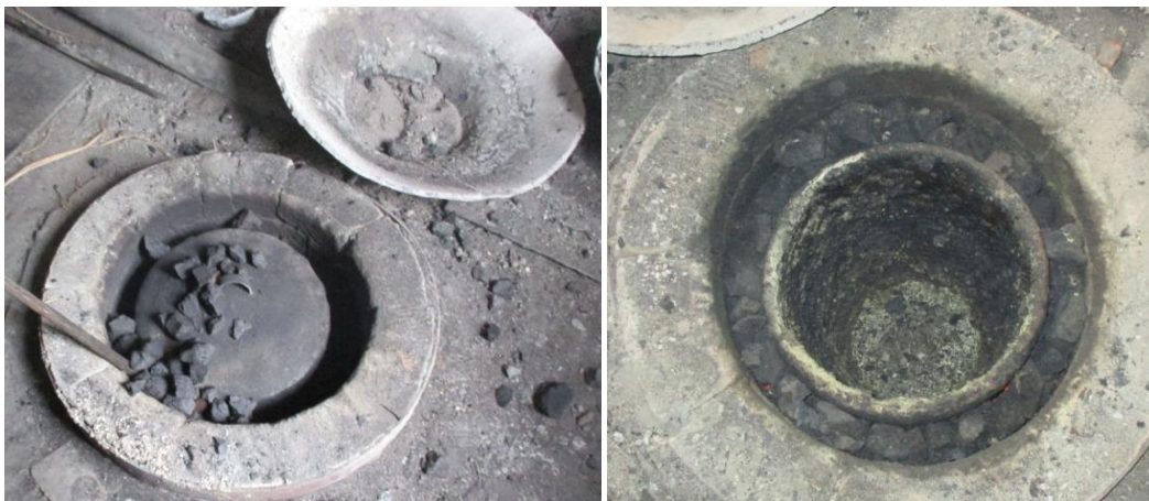
Figure 2.6: Filling of hard coke along the sides of crucible
