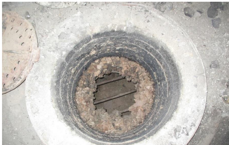
Figure 2.10: Inner view of pit furnace being used for scrap melting
