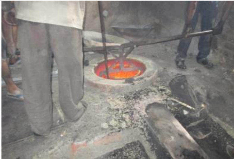
Figure 2.9: Removal of hot crucible at the end of operation
