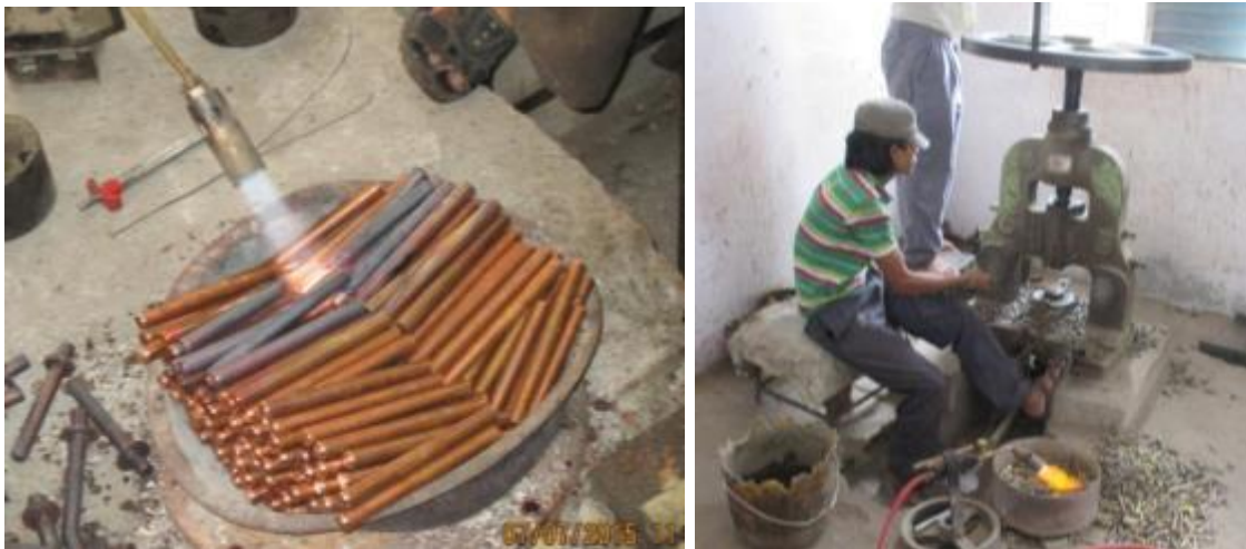
Figure 2.11: Heating of pieces using LPG before forging
