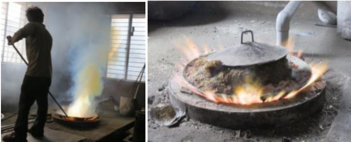
Figure 2.4: Melting of scrap in coke pit furnace
