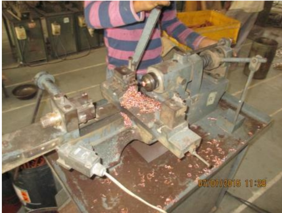
Figure 2.13: Machining operation for the production of nut bolt
