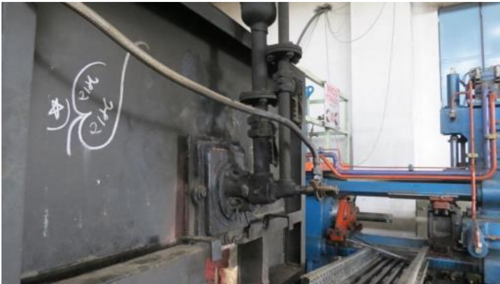
Figure 2.18: Pictorial depiction of billet reheating furnace
