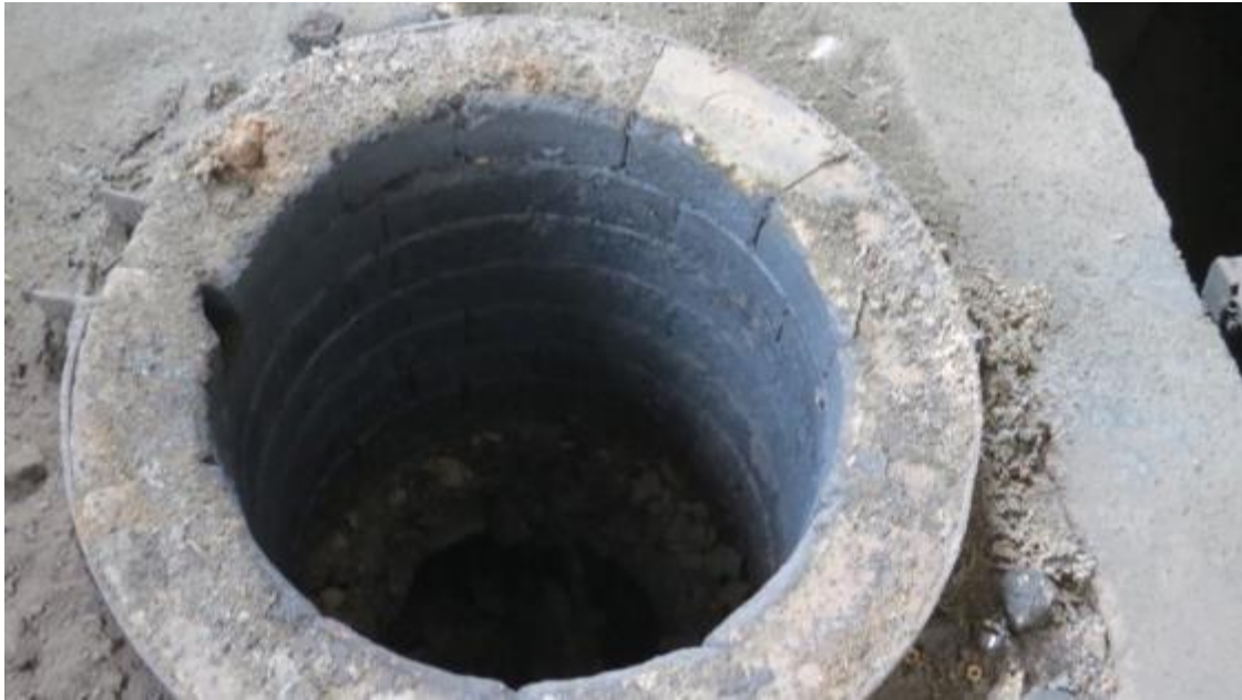
Figure 2.3: Inner view of coke Bhatti
