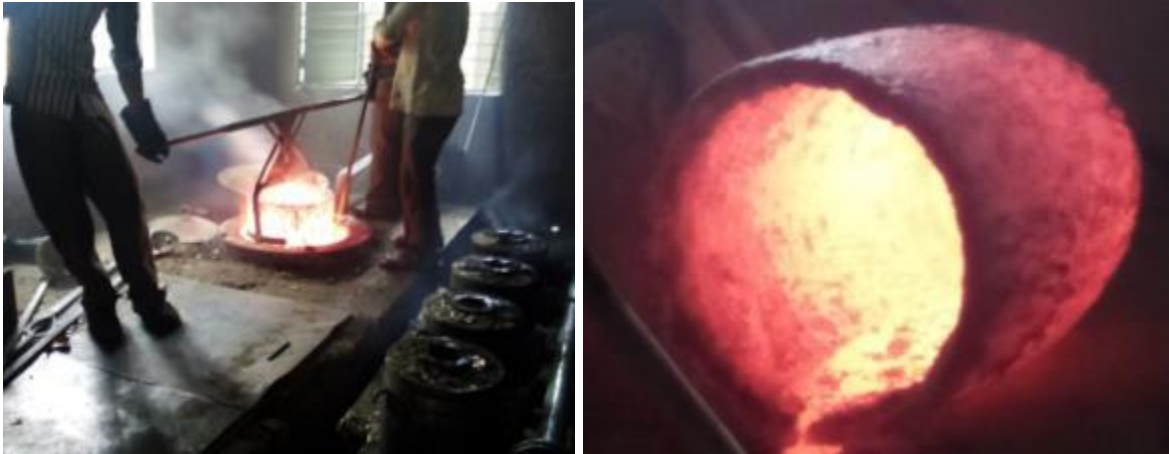
Figure 2.6: Removal of crucible from Bhathi at the end of operation
