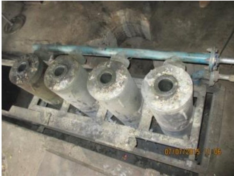
Figure 2.5: Dies ready for pouring of molten metal
