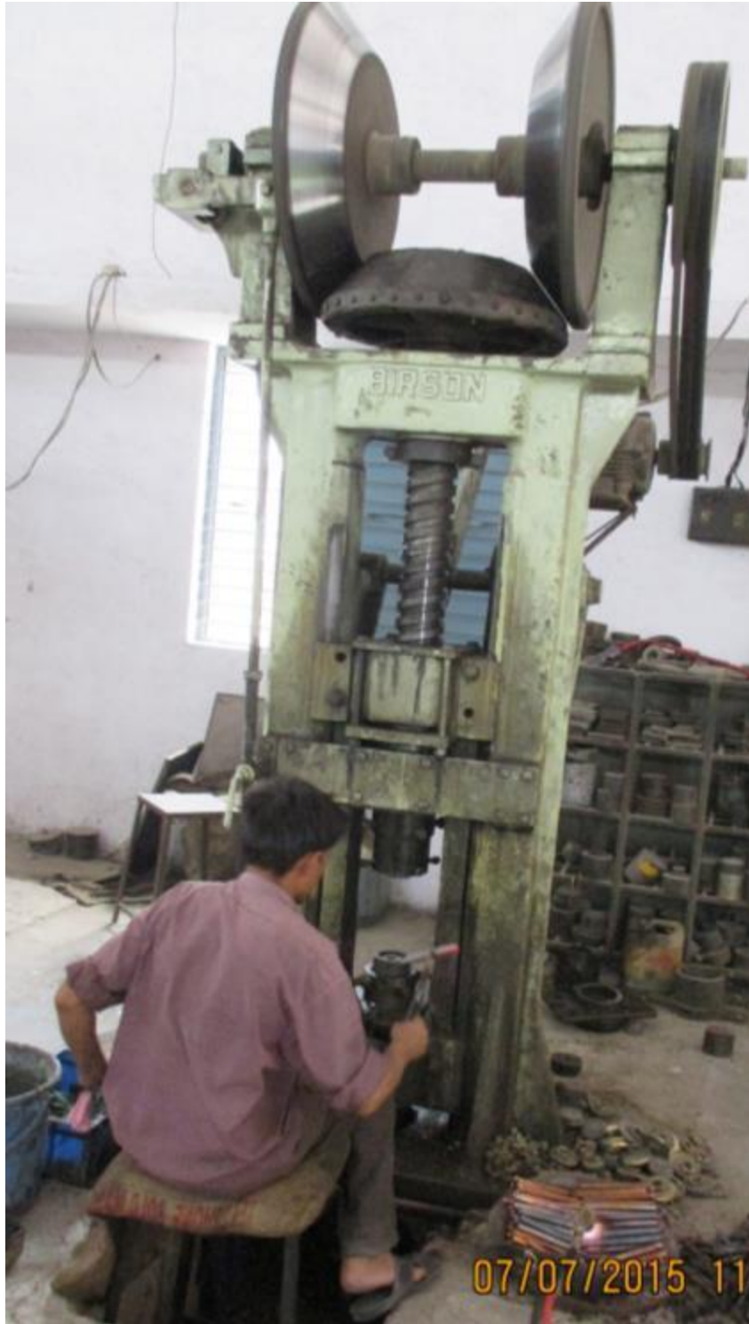
Figure 2.12: Forging press for production of bolts
