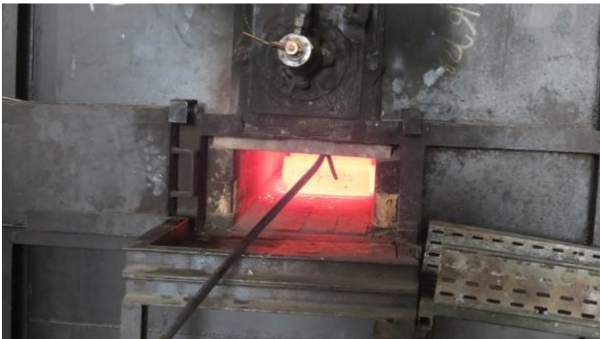
Figure 2.9: Hot billet coming out of furnace
