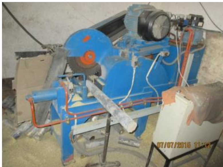
Figure 2.7: Circular saw machine for cutting of billets
