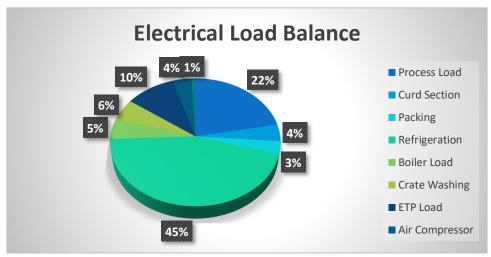
Figure 10: Equipment/Process wise energy breakup
