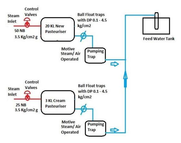
Figure 15: Schematic layout with trap installation
