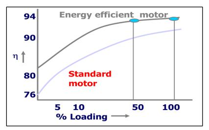
Figure 18: Loading Vs Efficiency curve
