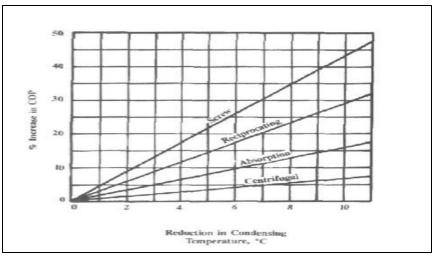
Figure 24: Effect of condensing temperature on COP
