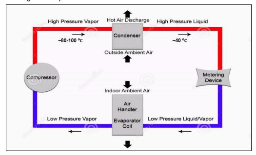
Figure 22: Vapor Compression Cycle
