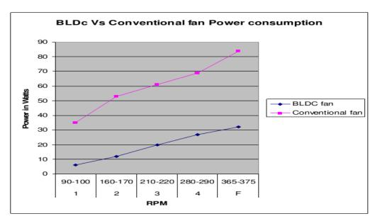
Figure 27: Comparison of normal fan vs BLDC fan
