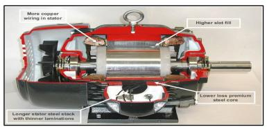
Figure 19: EE Motor features
