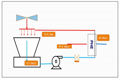
Figure 17: Schematic of PHE Condenser
