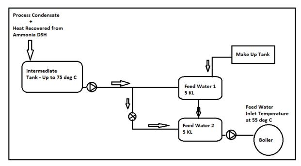
Figure 14: Schematic of hot water sources in the plant
