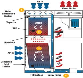
Figure 25: Evaporative condenser
