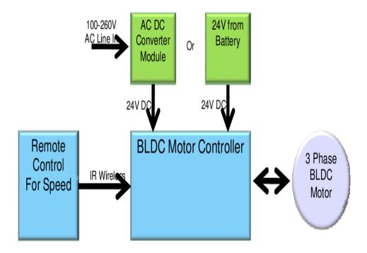
Figure 26: Schematic of BLDC fan
