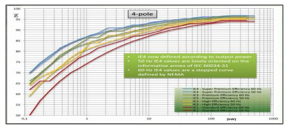
Figure 21: Losses in different classes of motors
