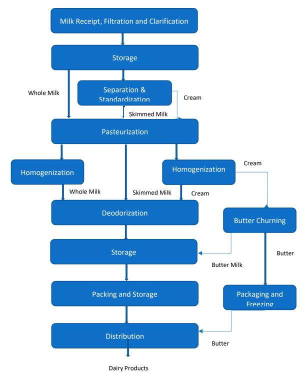
Figure 2: Typical process flow of Milk manufacturing
