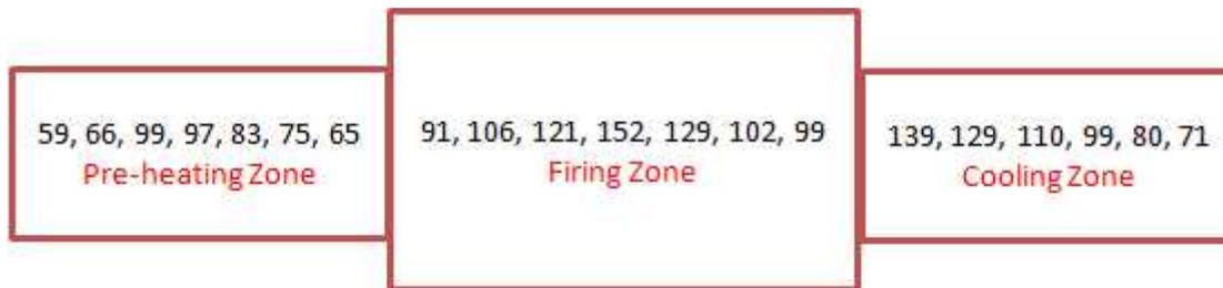
Figure 19: Measured skin temperature of kiln 2 (deg C)
