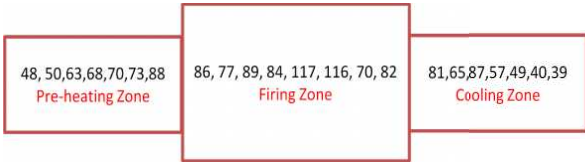
Figure 18: Masured skin temperatures of kiln (deg C)
