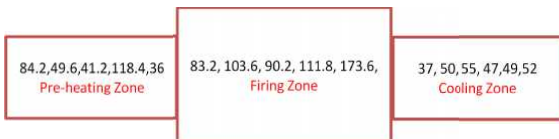
Figure 21: Measured skin temperatures of kiln (deg C)
