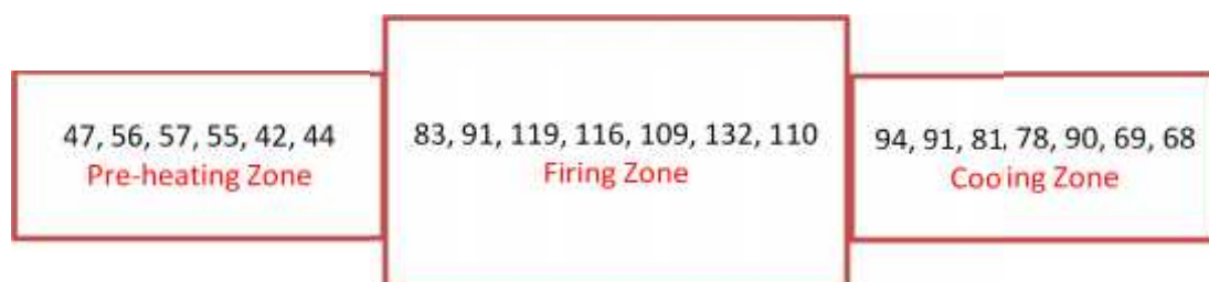
Figure 21: Measured skin temperature of kiln (deg C)
