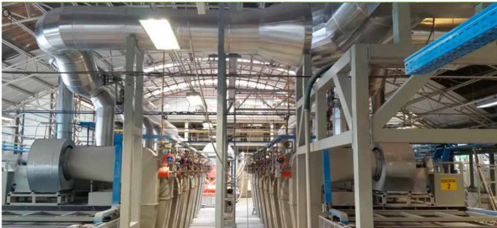
Figure 20: Heat recovery from kiln to dryer
