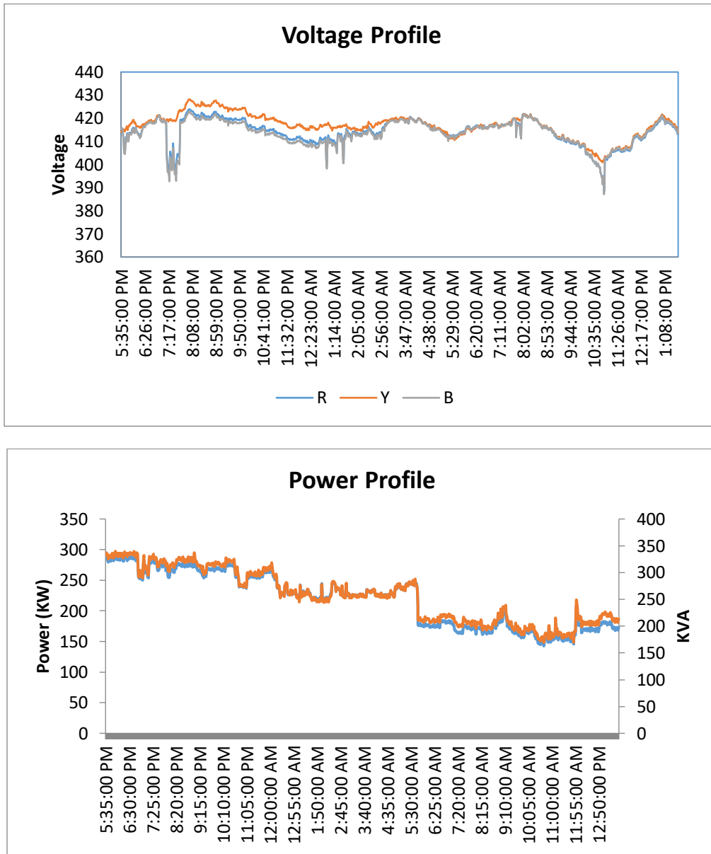
Figure 28: Power and voltage profile of Main Incomer
