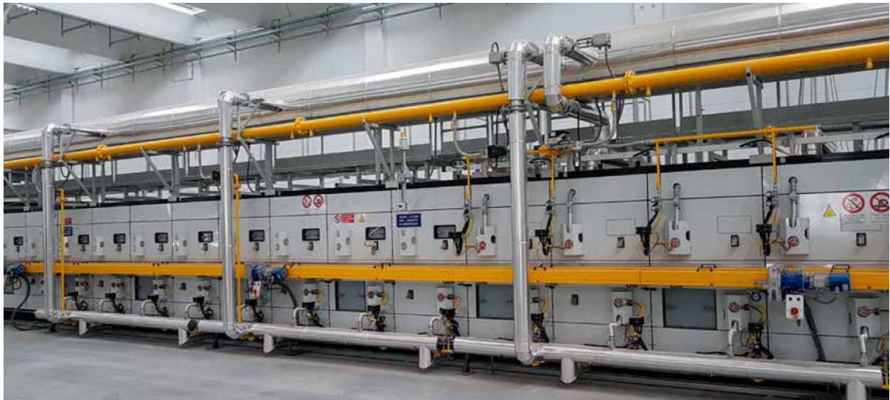
Figure 17 : Heat recovery system for combustion air
