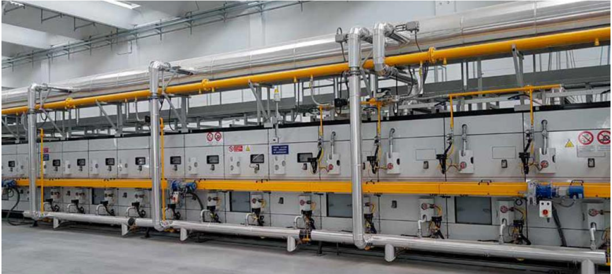
Figure 18 : Heat recovery system for combustion air
