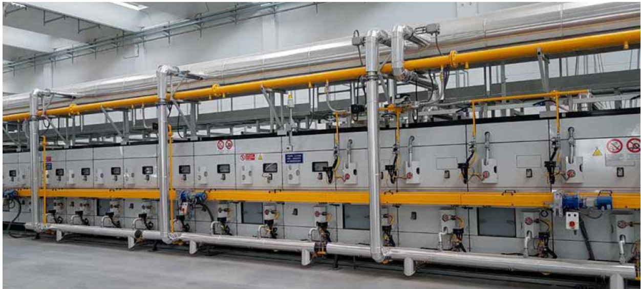
Figure 19 : Heat recovery system for combustion air
