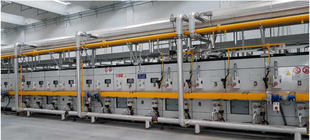
Figure 17 : Heat recovery system for combustion air
