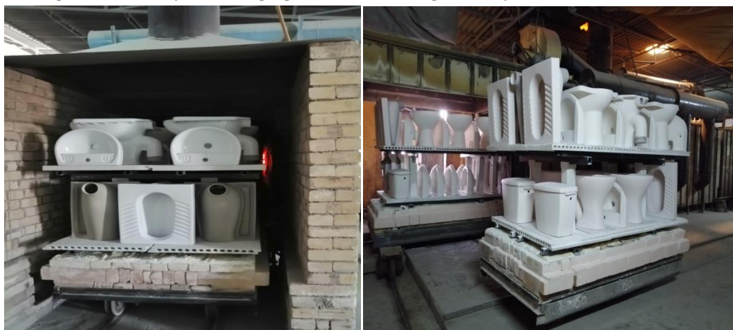
Figure 17: Pre drying and entrance of Tunnel Kiln
