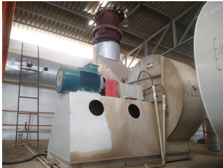
Figure 29: Direct drive blower fan
