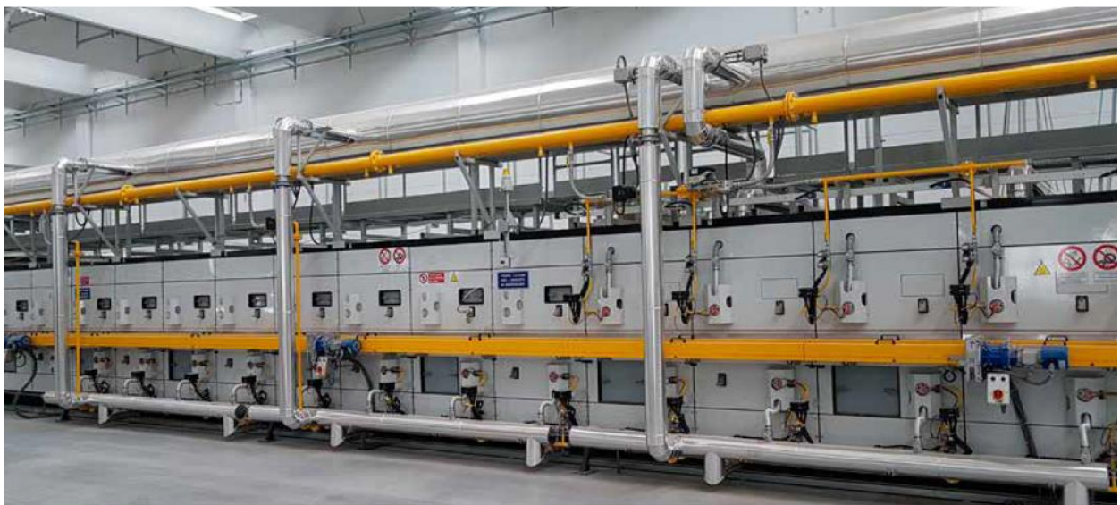
Figure 21: Heat recovery system for combustion air
