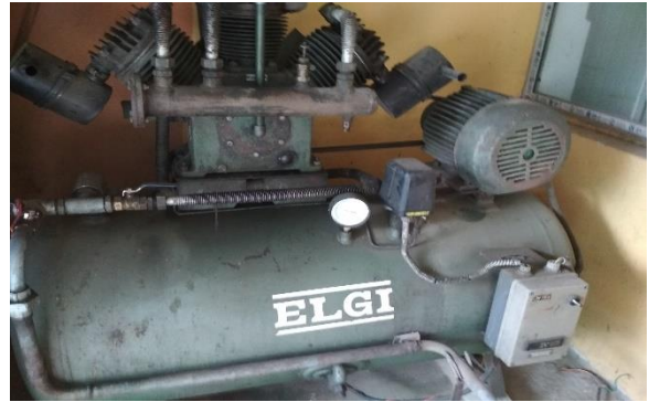
Figure 14: Old reciprocating compressor
