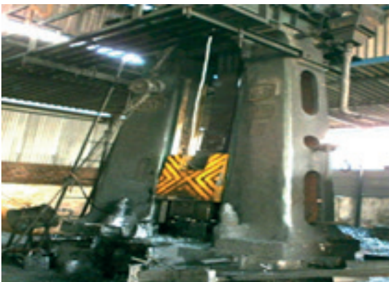
Closed-die hammer forging
