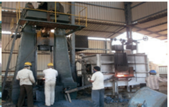
Closed-die hammer forging
