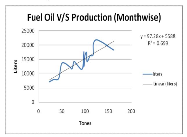
Average overall specific energy consumption is 173.5 liters/Ton out of which 97.3 liters per ton is variable. Considering that the theoretical requirement of heat for metal heating is not more than 20 Liters per ton, 80% of the heat from variable energy is wasted in stack losses which are proportional to the fuel firing( and finally production volume).
