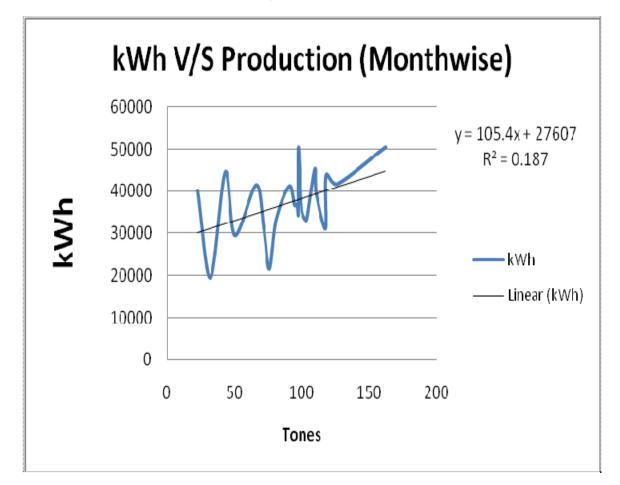
It is evident from the graph that the fixed electrical energy consumption is to the extent of 27607 kWh which is very high for lower production volumes. It is necessary to minimize fixed consumptions in electrical energy.
