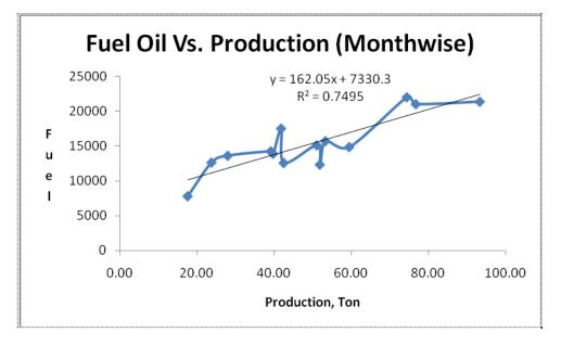
Average overall specific energy consumption is 341 liters/Ton. Considering that the theoretical requirement of heat for metal heating is not more than 20 Liters per ton, 85% of the heat from variable energy is wasted in stack losses which are proportional to the fuel firing( and finally production volume).
