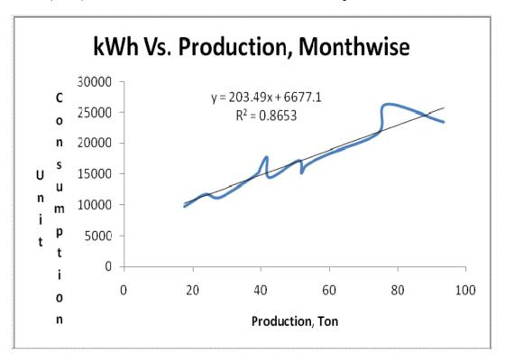
It is evident from the graph that the fixed electrical energy consumption is to the extent of 6671 kWh which is very high for lower production volumes. It is necessary to minimize fixed consumptions in electrical energy.
