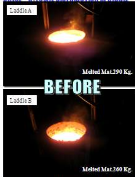
IMBALANCE METAL DISTRIBUTION BETWEEN LADDLES
