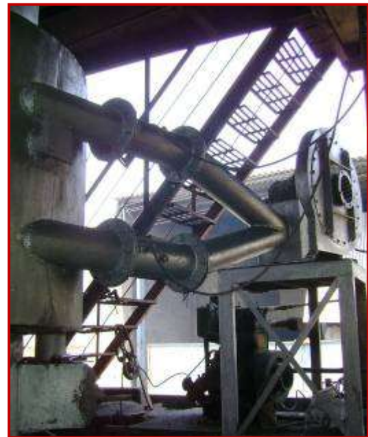
Figure 2.3(b): Divided blast mechanism in a cupola
