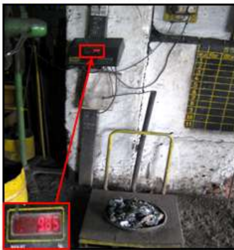
Slag generation from without shotblasted RR
