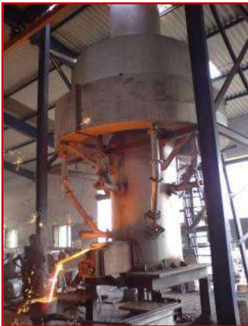
Figure 2.3(a): Cupola operation in a foundry
