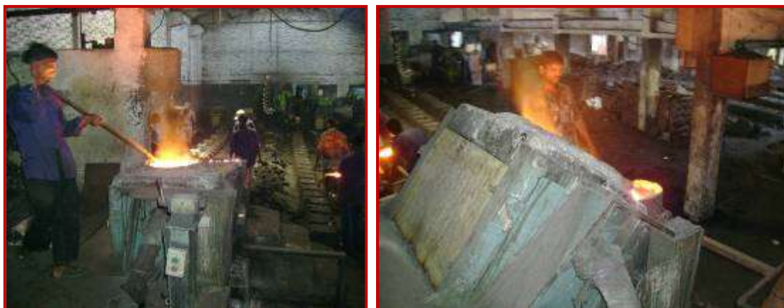
Figure 2.4: Induction furnace – melting and pouring operation
