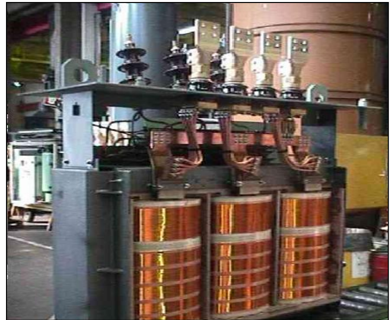
1600 kVA Amorphous Core Transformer
