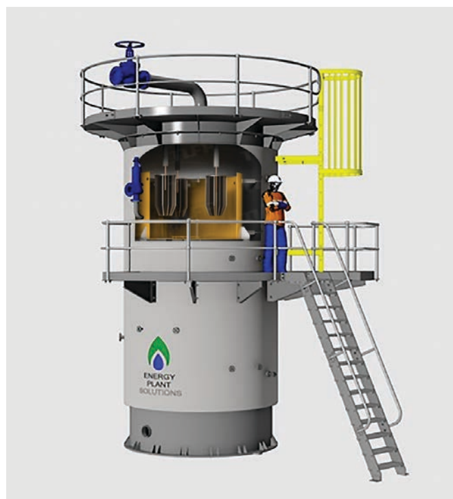
An example of an electrode boiler. Note the three electrode prongs that can be raised or lowered to create steam on demand.
