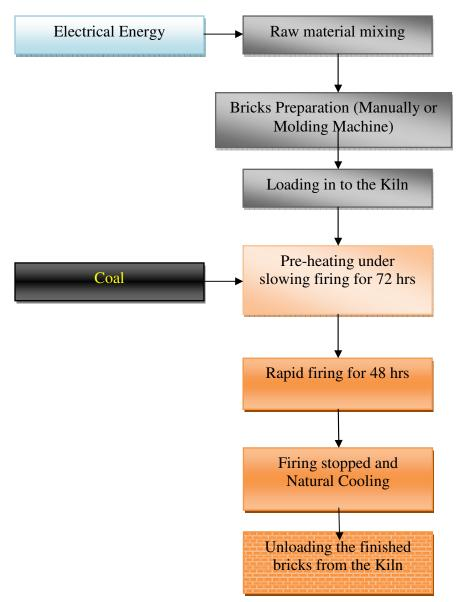
The Refractory Bricks manufacturing process consists of following process involved to complete the one batch production.
