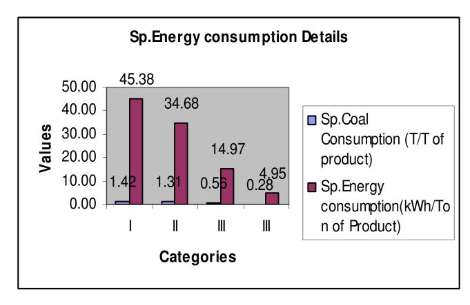
The total electrical energy consumption by 30 refractory Industries is about 8 lakhs kWh/ year, coal consumption is about 30581 MT/ year and total production is 45040 MT. **Note**: The energy consumption in the refractory Industries depends up on DD kiln efficiency, % utilization and type of products manufactured.
