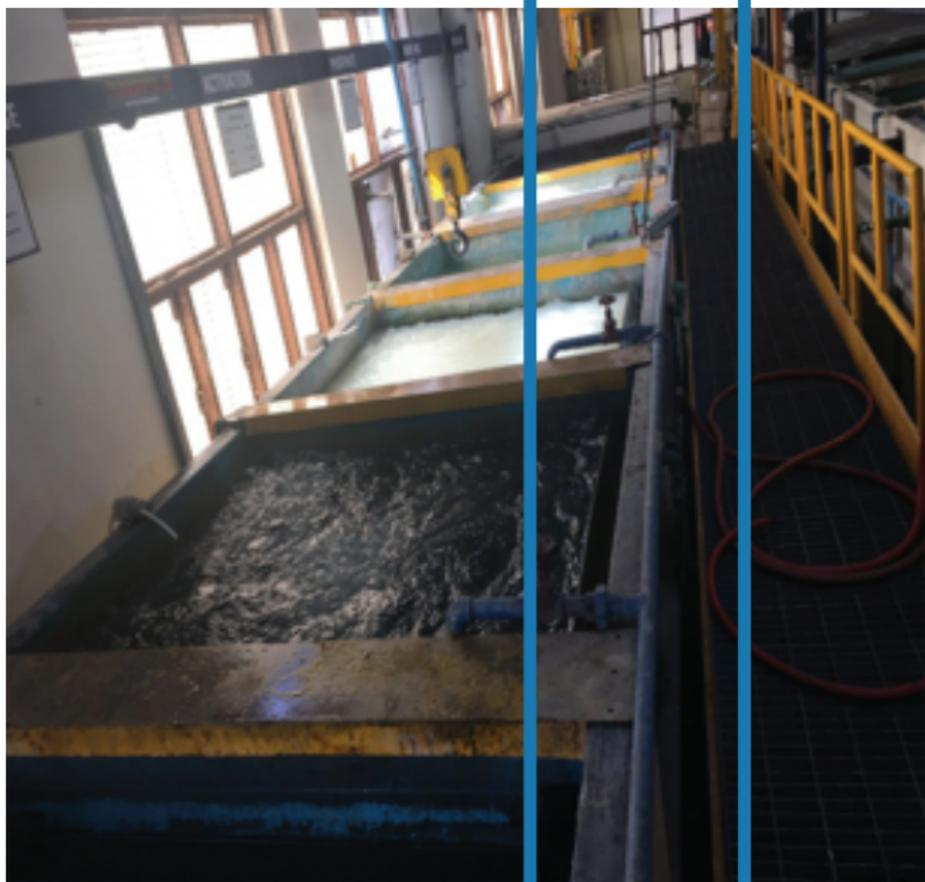
High Pressure Compressed Air Using @ 7 kg/cm<sup>2</sup> for Agitation
