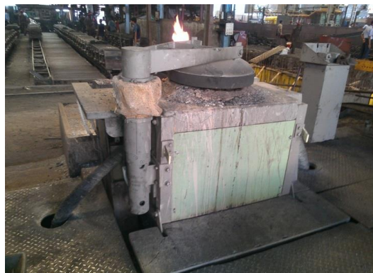
Lid mechanism for induction furnace crucible
