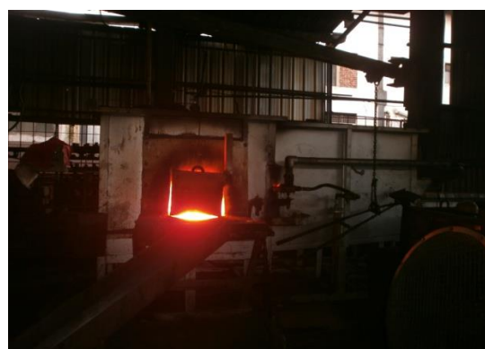
Radiation losses thorough door opening
