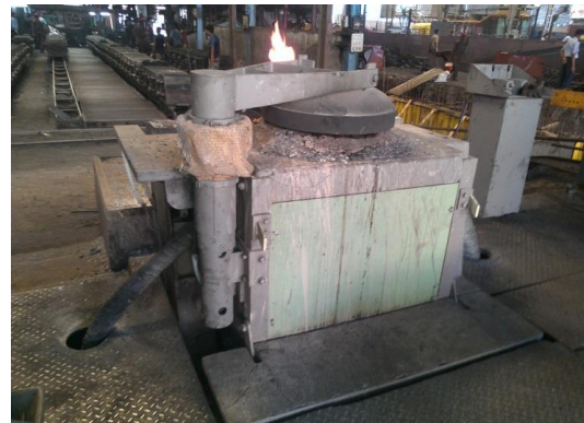
Lid mechanism for induction furnace crucible
